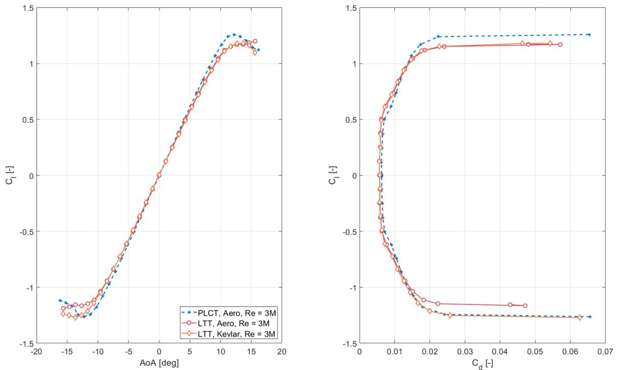
Figure 13: The lift vs. angle of attack and lift vs. drag polars of the NACA63018 in clean configuration.
