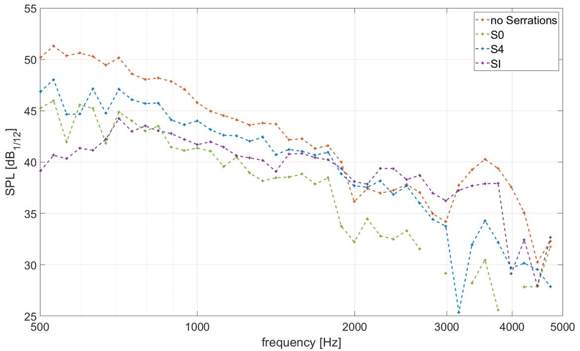
Figure 16: TE Noise spectra of the NACA63018 at 0 deg. angle of attack and Reynolds number 3 million for different serrations measured in PLCT.
