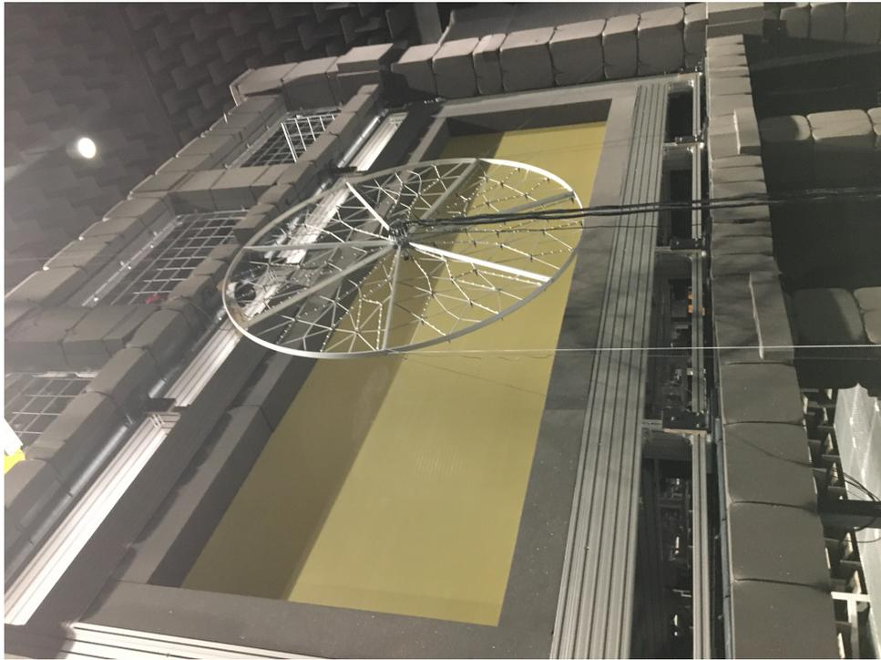
Figure 7: The microphone array and Kevlar wall.
