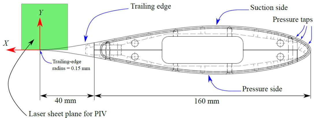
Figure 3: The small NACA63-018 aerofoil model.
