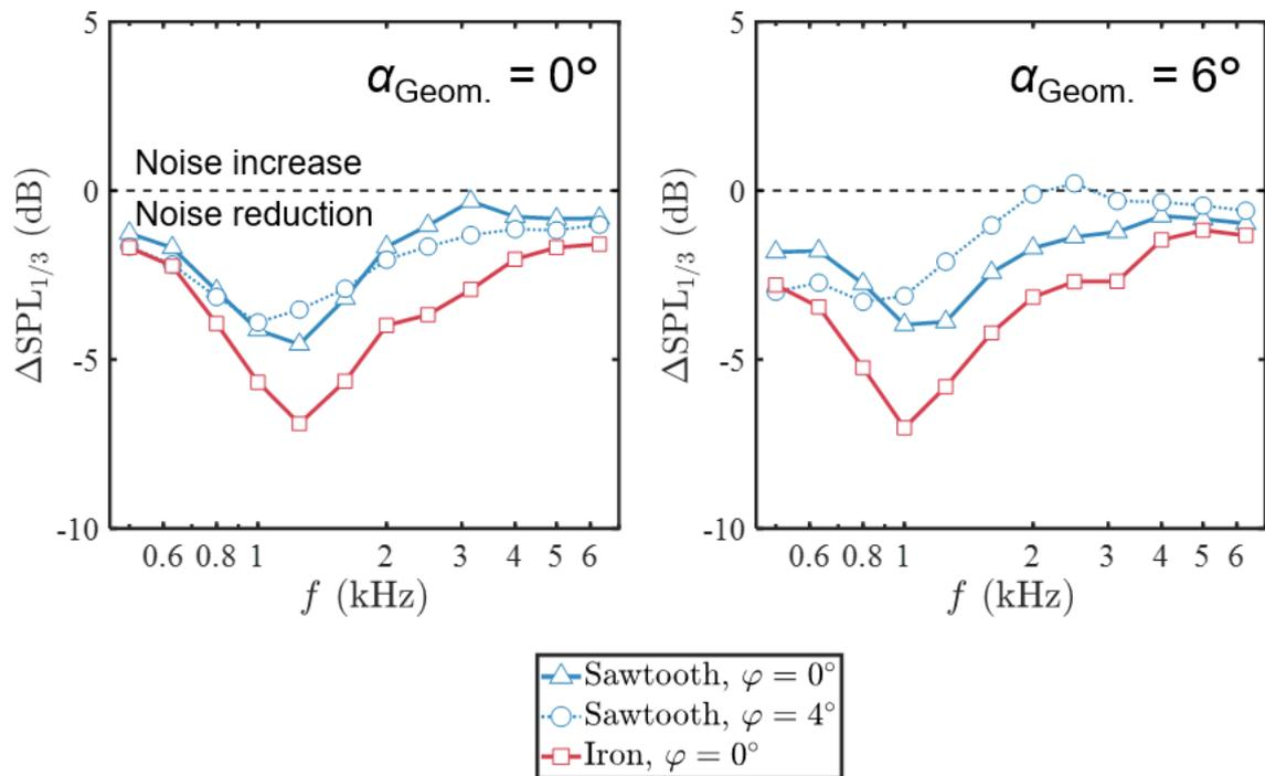
Figure 17: TE Noise reduction at Reynolds number 0.39 million with respect to the NACA63018 without serrations measured in the A tunnel.
