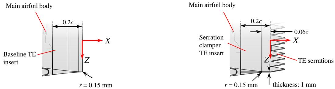
Figure 4: The serrations for the small model.
