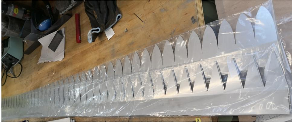
Figure 2: The extensions with serrations for the large NACA63-018 aerofoil model.
