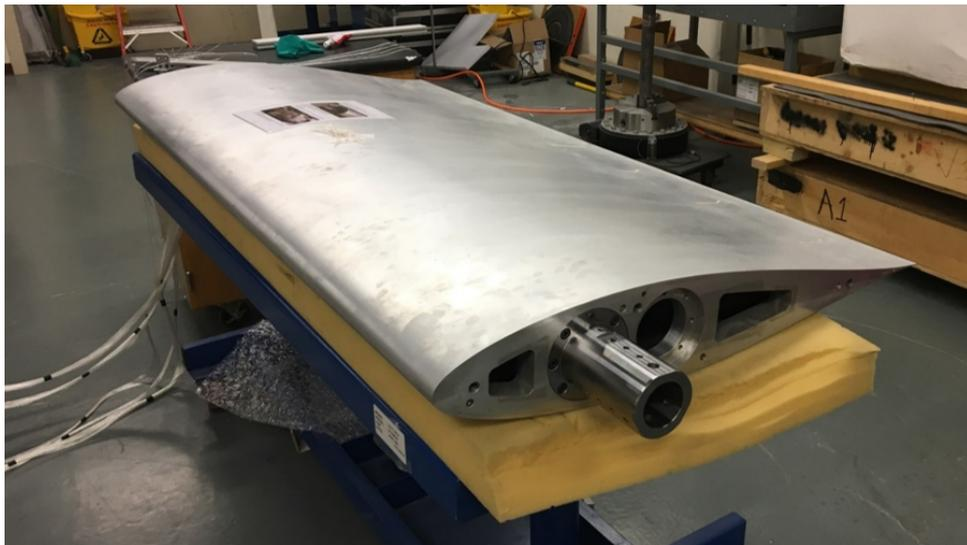
Figure 1: The large NACA63-018 aerofoil model.
