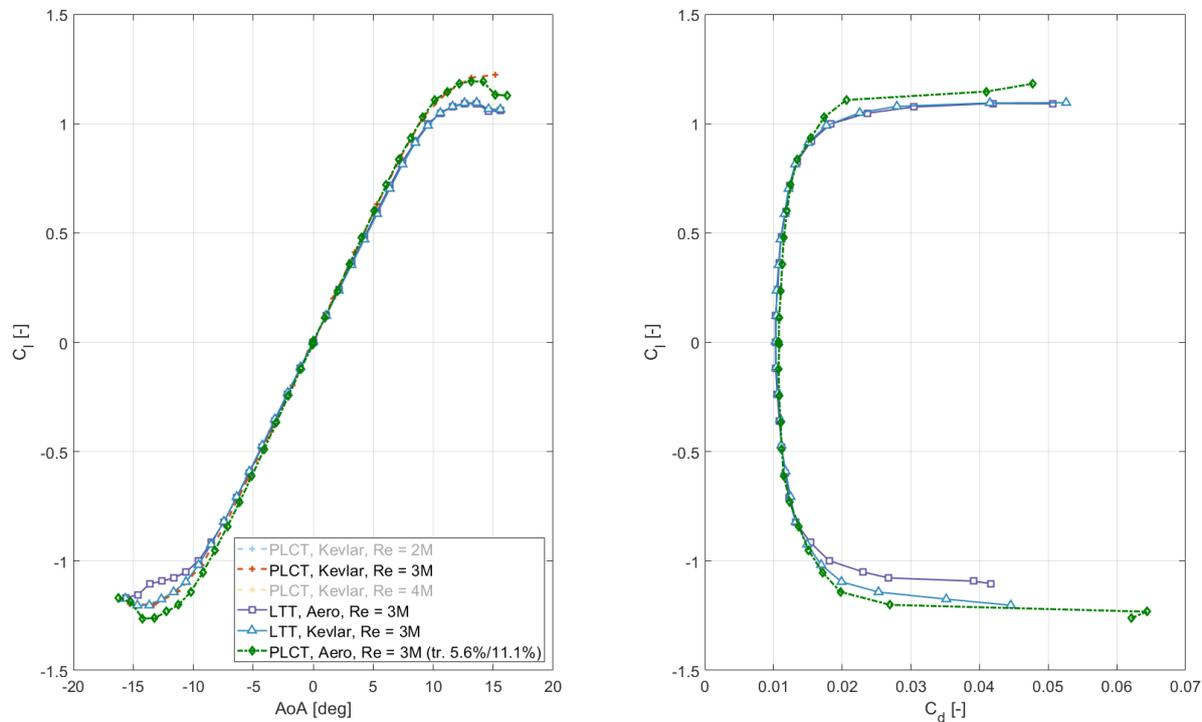
Figure 14: The lift vs. angel of attack and lift vs. drag polars of the NACA63018 in tripped configuration.
