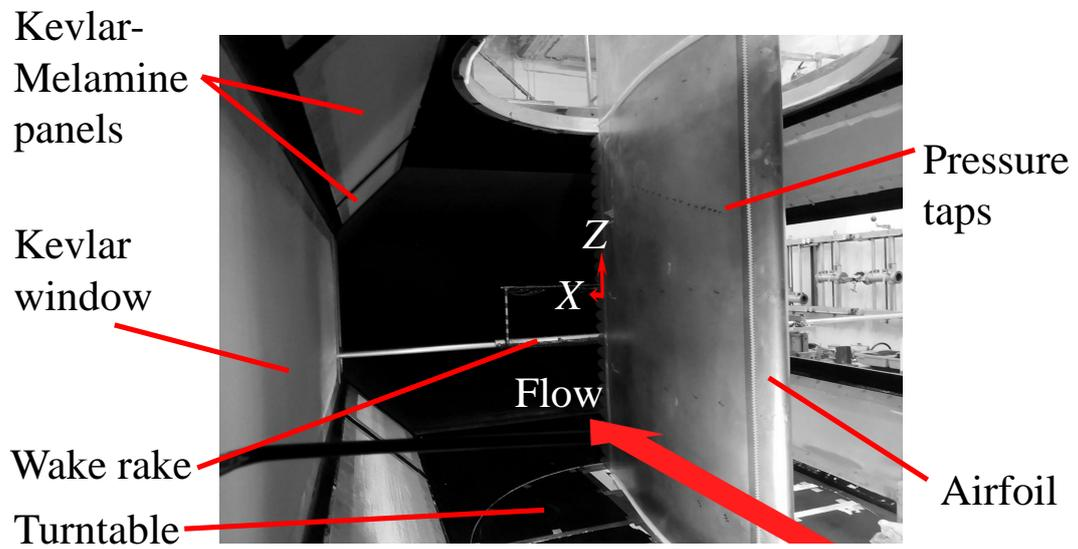
Figure 10: Acoustically treated test section for the LTT.
