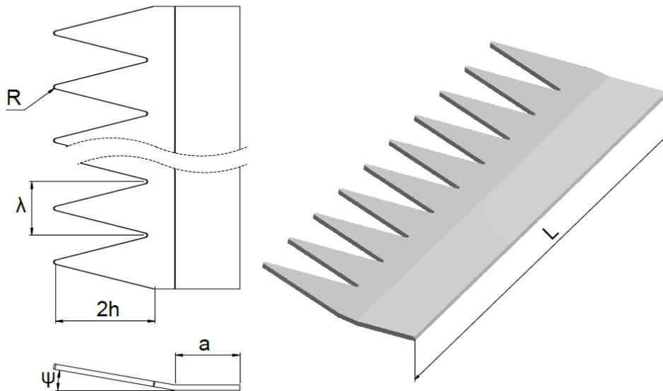
Figure 5: Definition of the design parameters for the serration geometries.
