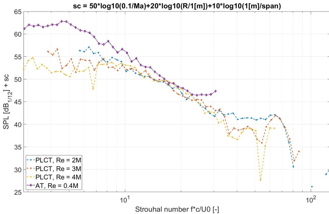
Figure 15: TE Noise spectra of the NACA63018 at 0 deg. angle of attack in tripped configuration without serrations.
