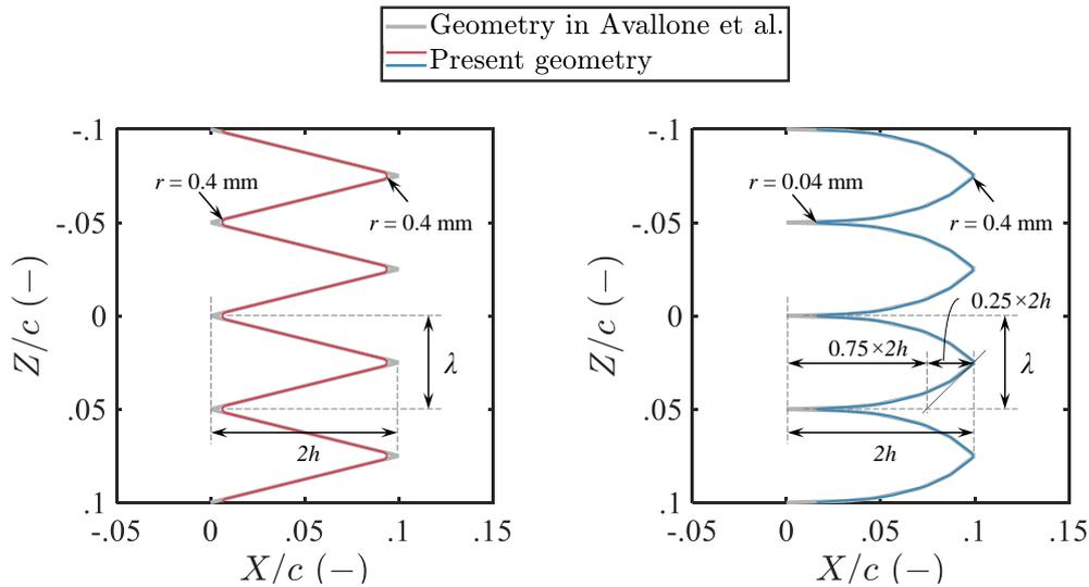
Figure 6: The theoretical serration geometry.
