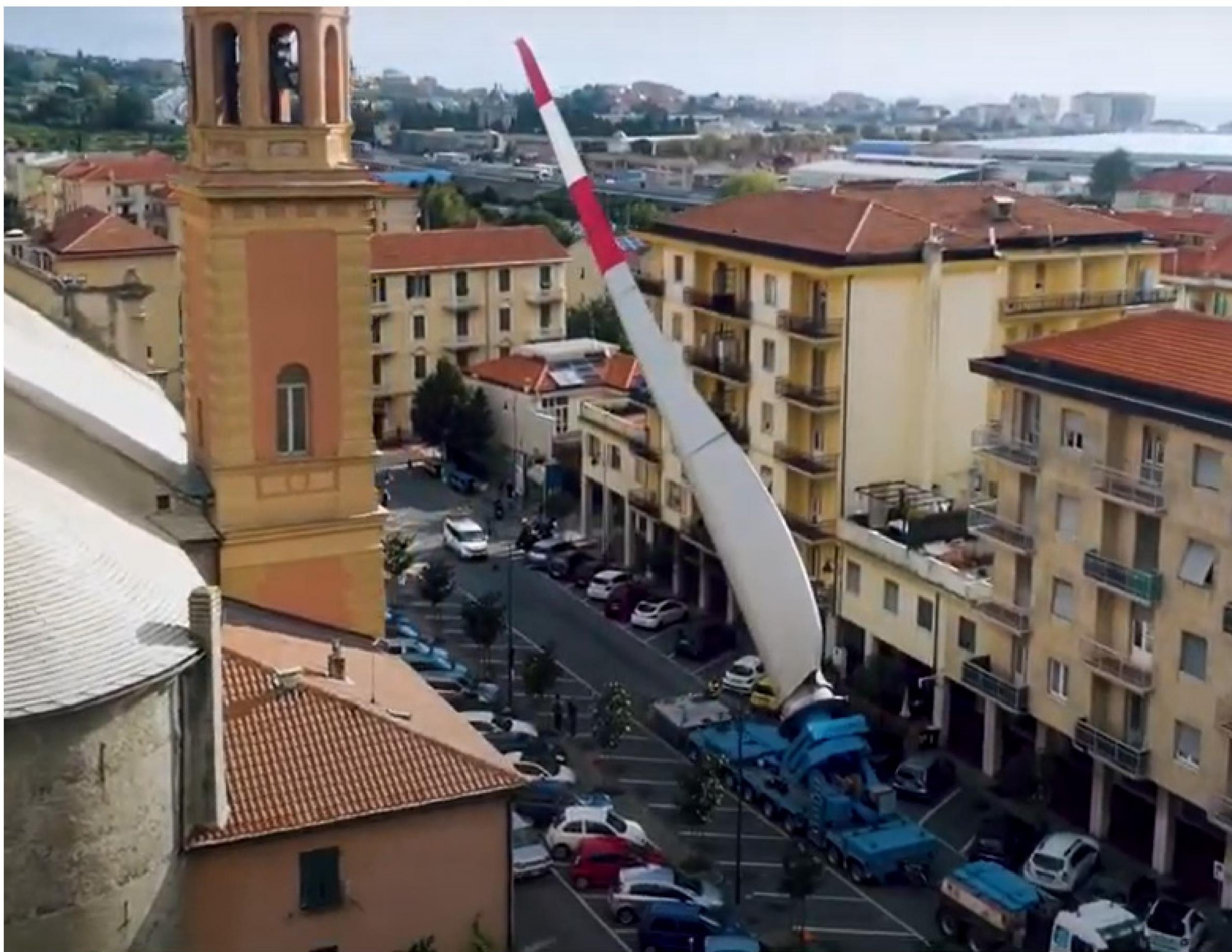
OPENING PHOTO: BLADE TRANSPORT WITH INNOVATIVE BLADE LIFTER SYSTEM THROUGH A SMALL VILLAGE IN LIGURIAN REGION TO THE SITE OF INSTALLATION OF ROCHE BIANCHE WIND PLANT .(CREDITS: PHOTOGRAPH MARCO RIMONDI AND COPYRIGHT FERA SRL, WWW.FERASRL.IT )
