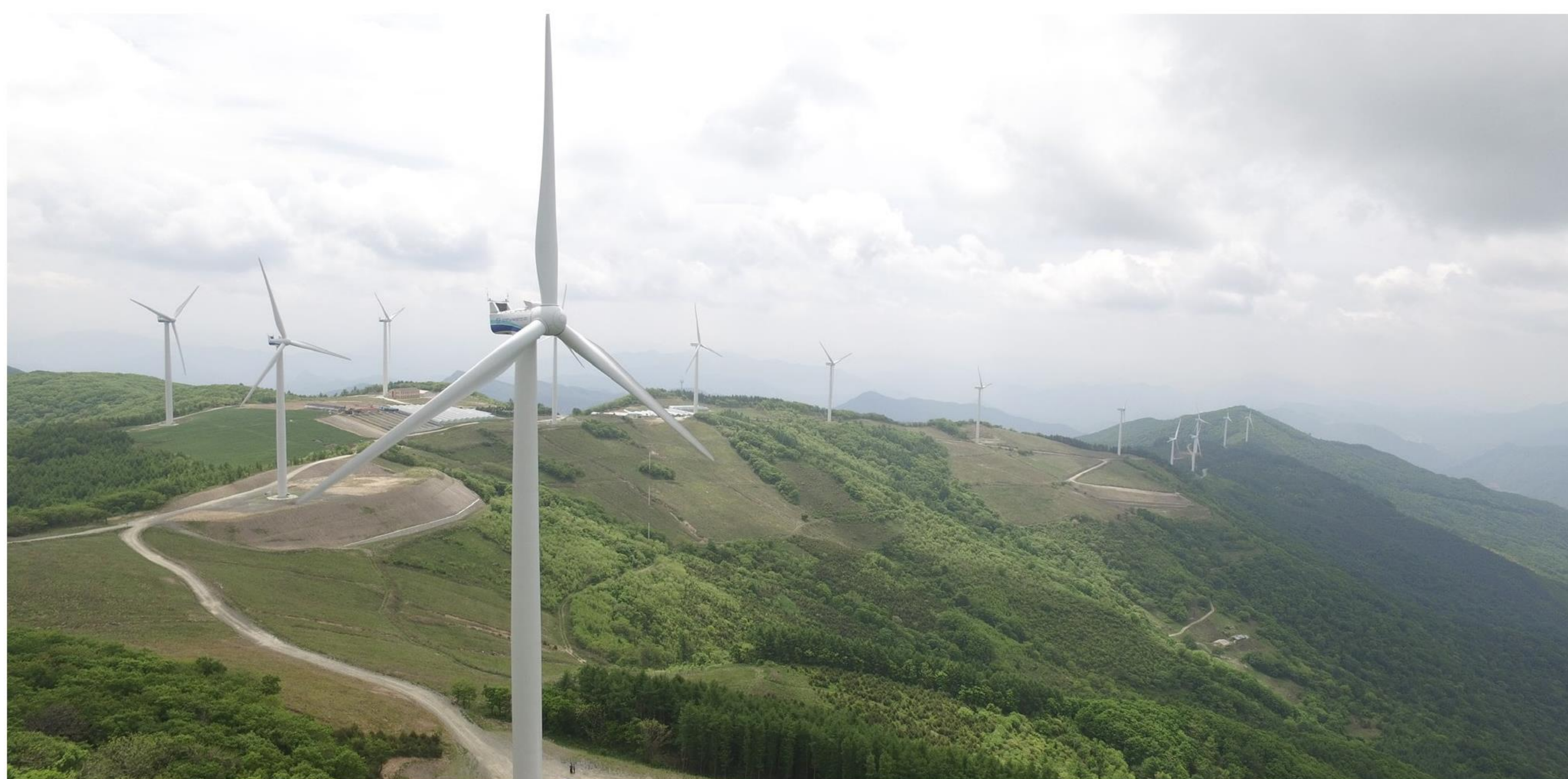
[PHOTO 3] PYEONG-CHANG WIND FARM, GANGWON-DO, KOREA, HYOSUNG 2MW AND HYUNDAI HEAVY INDUSTRY 2MW WTGS, SOURCE: KOREA SOUTHERN POWER CO., LTD.
