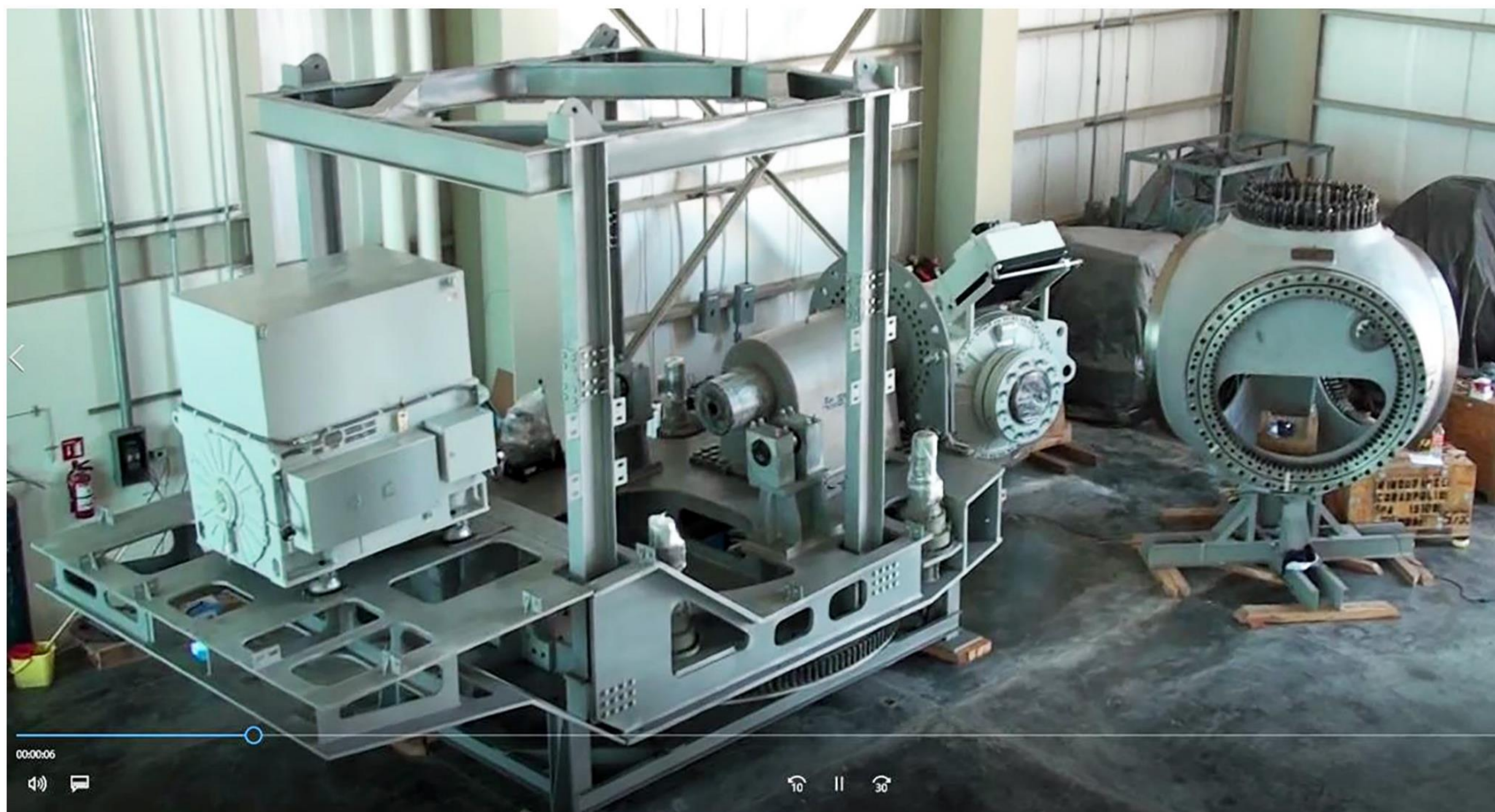
FIGURE 2: POWER TRAIN OF A PROTOTYPE 1.2 MW WIND TURBINE (PHOTO CREDIT: © CEMIE-EÓLICO).
