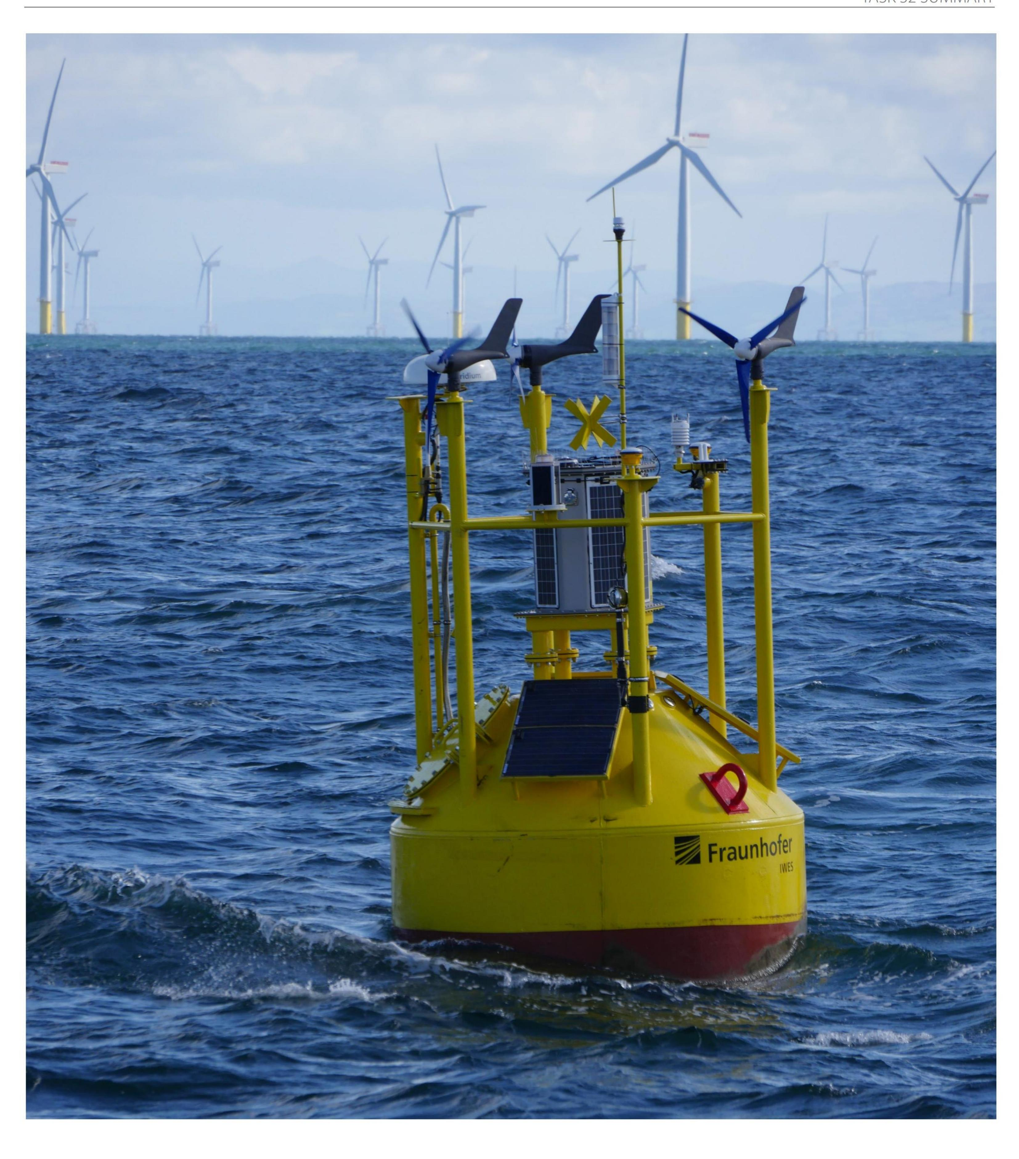
It is very difficult to get accurate, long-term wind resource measurements in cold climates using traditional met towers. These are vulnerable to icing and require power supplies for continuous operation. By contrast, wind lidar are often simpler to maintain
