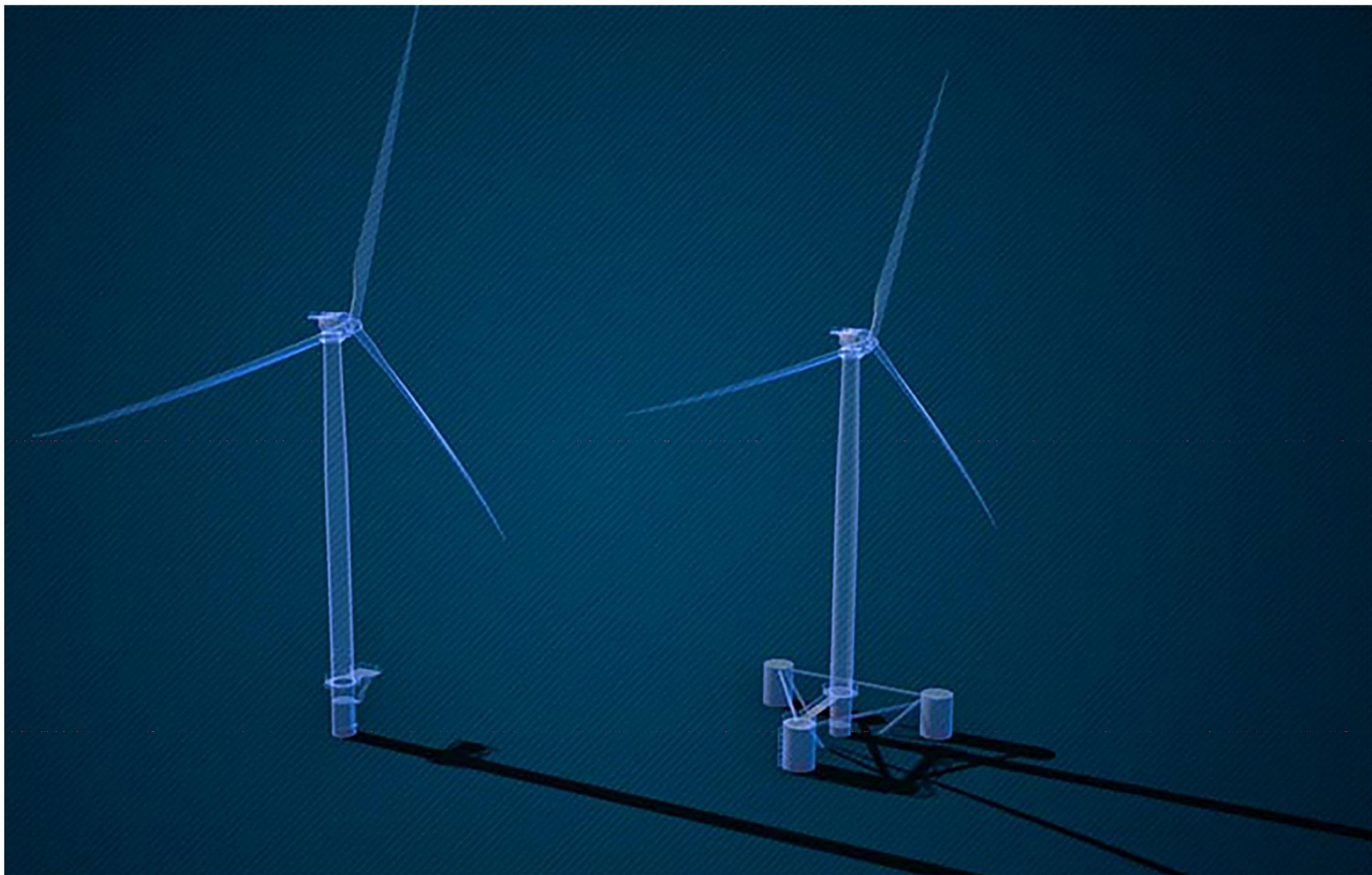
FIGURE 2: THE IEA WIND 15-MW REFERENCE WIND TURBINE (GRAPHIC: JOSHUA BAUER, NATIONAL RENEWABLE ENERGY LABORATORY)
