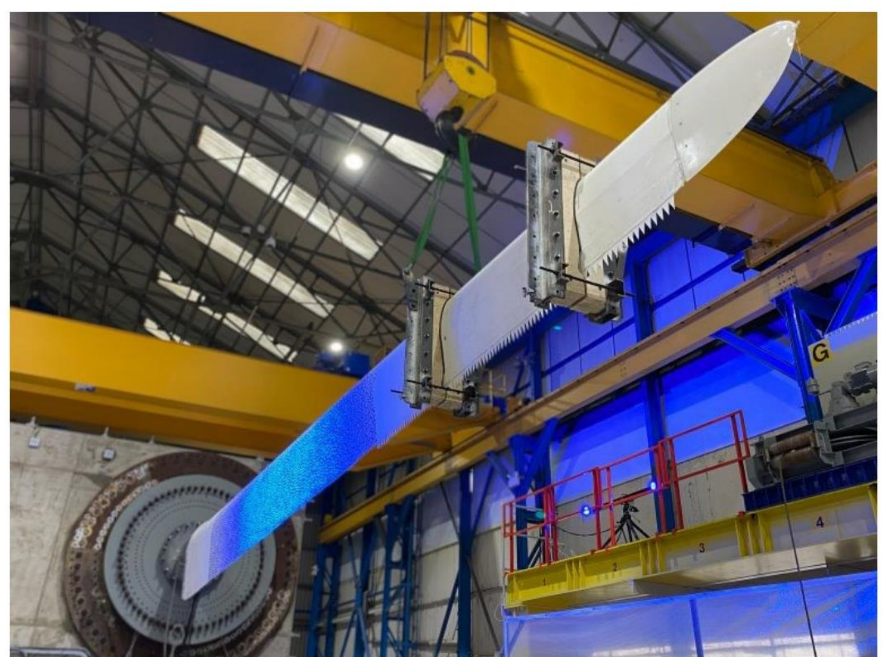
ACT BLADE GRAPHIC (LEFT) AND TESTING AT THE NATIONAL RENEWABLE ENERGY CENTRE, BLYTH (RIGHT) (SOURCE: ACT BLADE (L), ORE CATAPULT (R))
