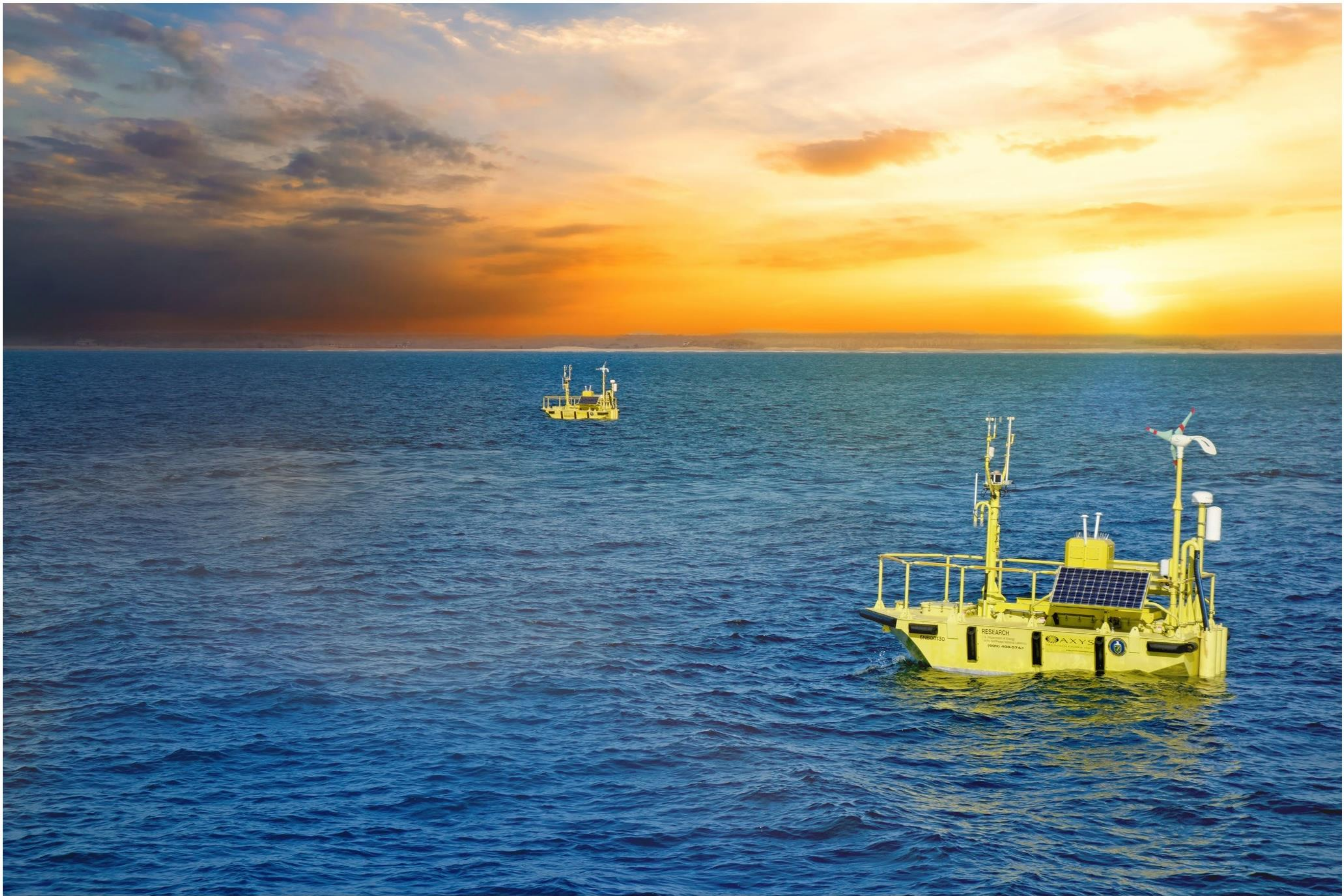
FIGURE 1. PACIFIC NORTHWEST NATIONAL LABORATORY (PNNL) RESEARCHERS UPGRADED THE INSTRUMENTATION ON TWO LIDAR BUOYS USED TO CAPTURE DATA AT NEARLY TWICE THE HEIGHT OF PREVIOUS INSTRUMENTATION, HELPING MEET THE DATA NEEDS FOR TODAY'S MUCH TALLER WIND TURBINES. IMAGE: OCEAN TECH SERVICES AND PNNL
