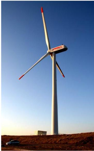
Figure 5 SUBARU 80/2.0 prototype 2 MW downwind turbine
