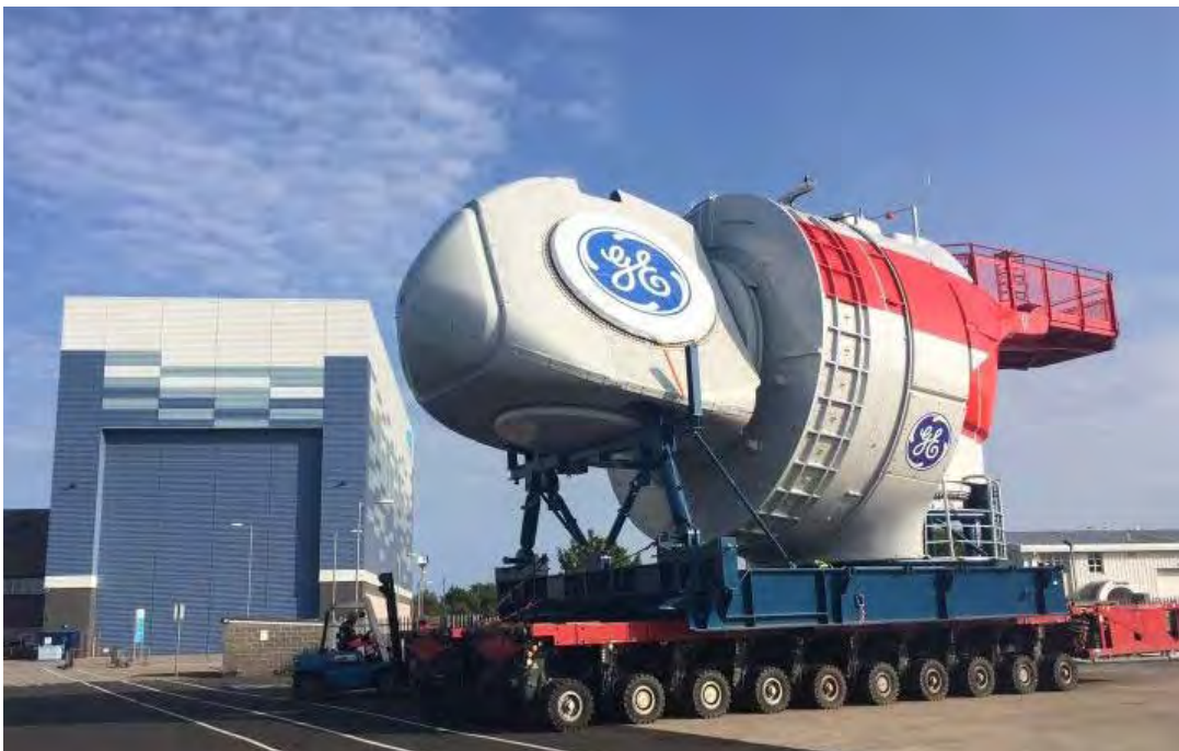
Figure 3. GE's Haliade 150-6 MW nacelle arrives in ORE Catapult's Blyth facility (Source: ORE Catapult)
