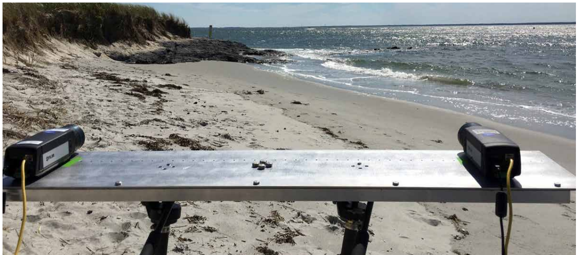
Figure 1. Two cameras equipped with ThermalTracker software designed to capture the flight patterns of birds and bats and provide more accurate data about their behavior around offshore wind turbines. (Photo courtesy of PNNL)
