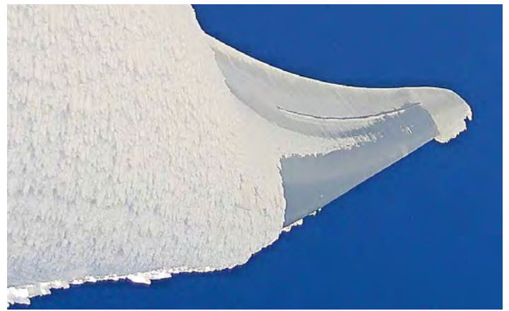
Figure 1. Icing observed on wind turbine blade (Photo credit: Nergica)
