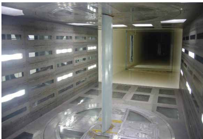
Figure 2. The photos of the refrigeration experiment of the Goldwind HQ63-17 airfoil in tunnel
