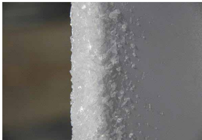
Figure 2. The photos of the refrigeration experiment of the Goldwind HQ63-17 airfoil in tunnel
