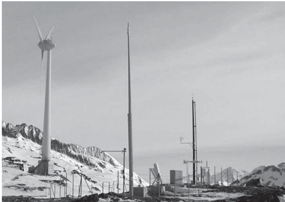
Figure 8 Alpine Test Site Gütisch, with a mit einer 600-kW wind power plant as well as a device for testing different measuring instruments under cold and icy conditions.
