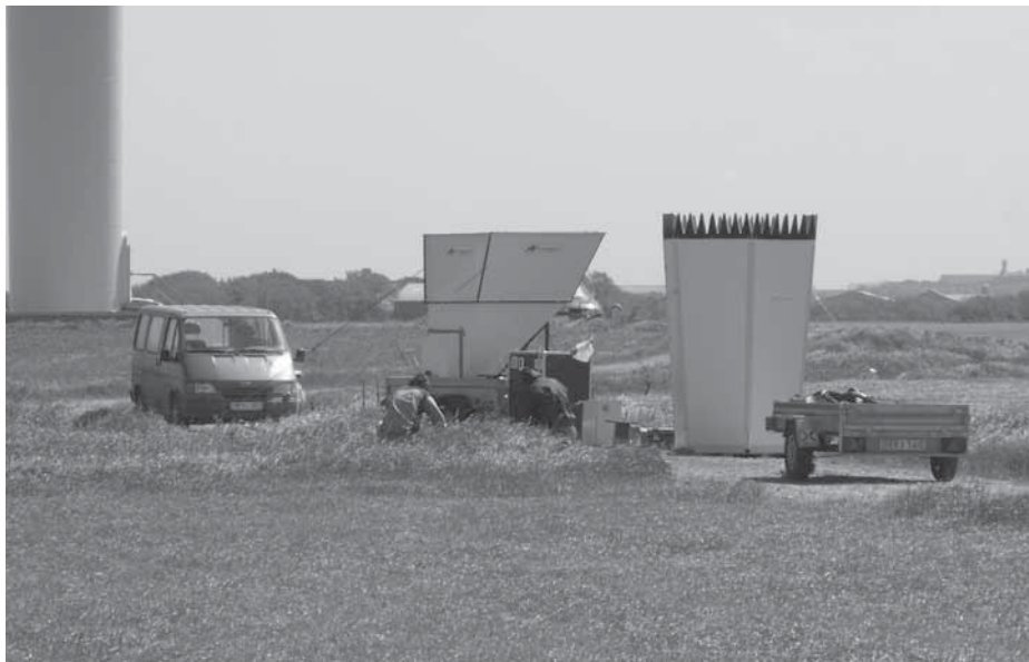
Figure 8 A SODAR installation at the test site for MW-sized wind turbines at Høvsøre. The wind field is measured up to a height of 150 m.
