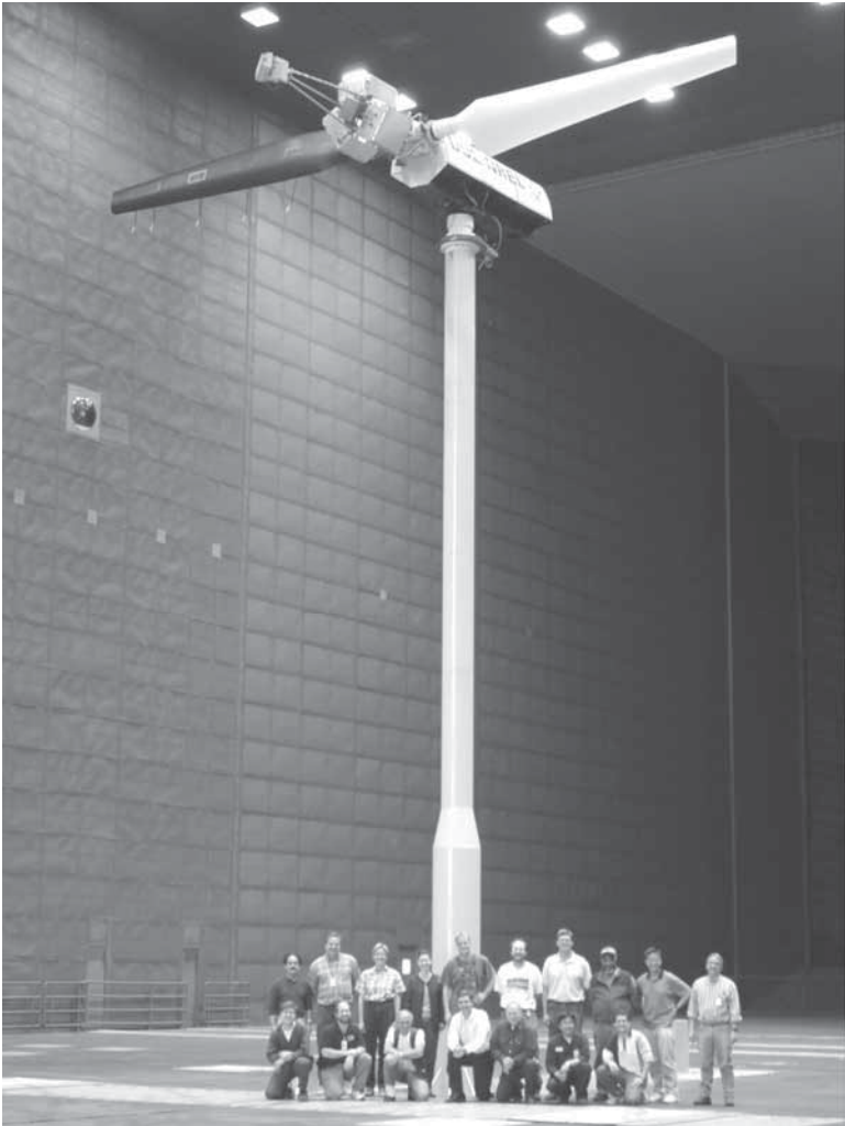
Figure 1 NREL Unsteady Aerodynamics Experiment wind turbine in NASA Ames 80 foot by 120 foot wind tunnel.
