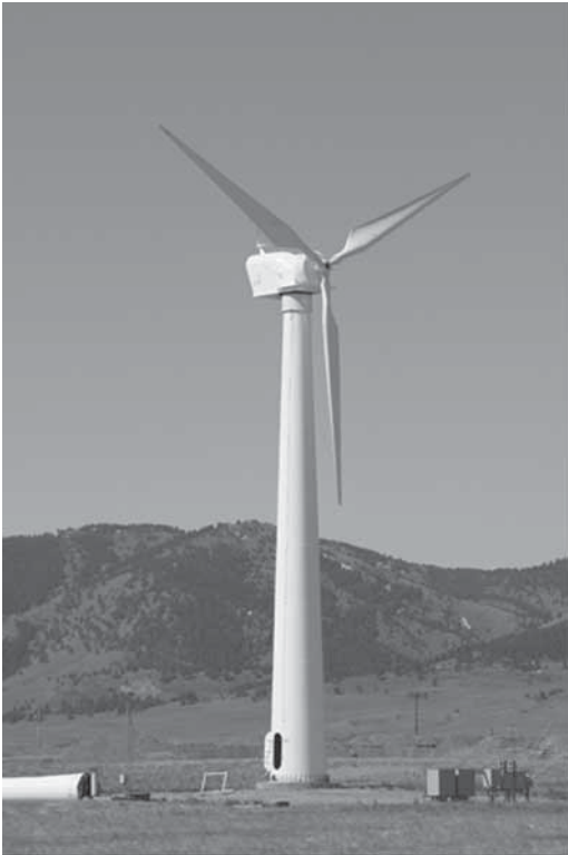
Figure 7 Northern Power Systems' new 100-kW machine will undergo loads, power quality, and acoustic emissions tests at the NWTC in 2008.
