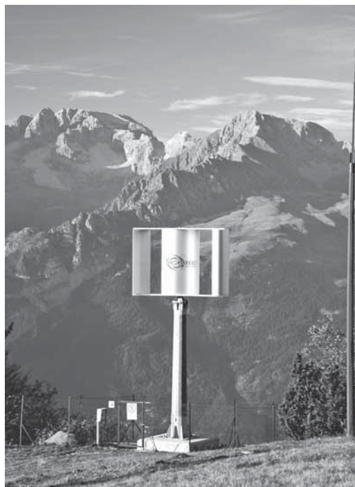
Figure 7 A Ropatec small-sized vertical-axis turbine on Monte Casale in the Italian Alps near Trento (courtesy of Ropatec).
