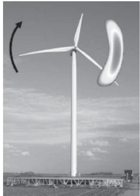
Figure 11 Picture of test set-up for acoustic measurements on the GE baseline turbine. The distribution of noise sources in the rotor plane is projected onto the picture.
