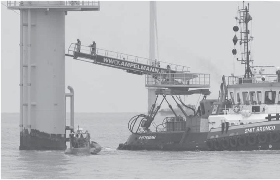
Figure 6 First personnel transfer with Ampelmann Demonstrator onto turbine of OWEZ. Photo: Jos Beurskens, We@Sea.
