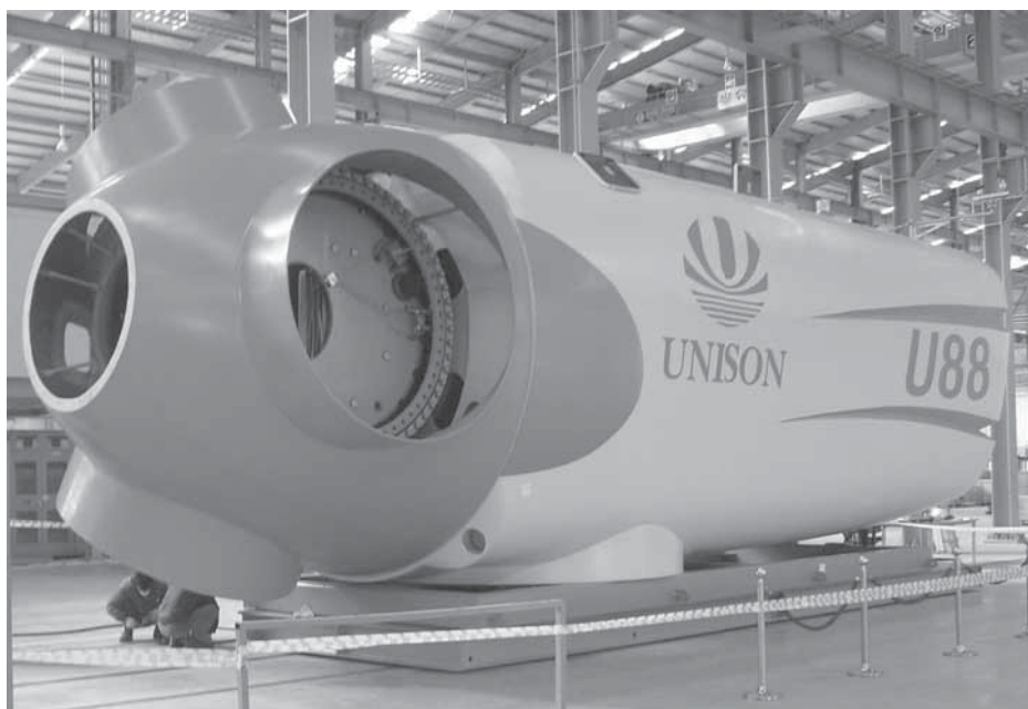
Figure 1 The Prototype of Unison's 2-MW PMSG wind turbine, U88.
