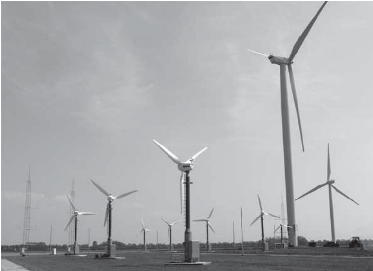
Figure 7 Scaled wind farm at ECN test site. Photo: Jaap 't Hooft, Senter-Novem.
