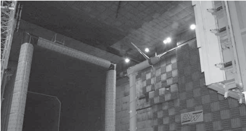
Figure 1 The MEXICO model turbine in the LLF tunnel of DNW. The blue box is the yawable balance and the (vertical) yaw axis passing through the rotor center. The tunnel collector is shown in the background and the nozzle in the foreground. The nozzle measures 9.5 m 2 , the collector 9.7 m 2 .
