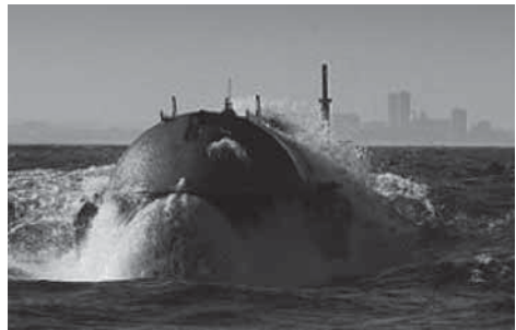
Figure 13 The front of the PELAMIS machine at the Aguçadoura Wave Park with the city of Póvoa de Varzim in the background (5).
