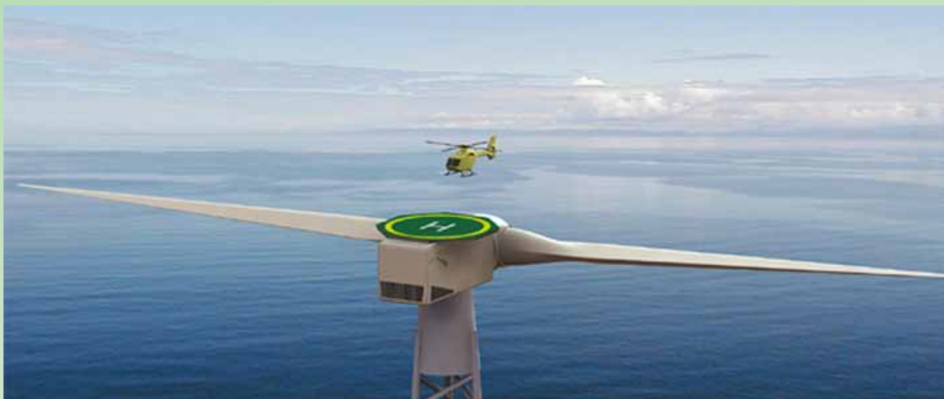
Figure 4 Artist impression of the 2-bladed 6-MW downwind turbine of 2B-Energy
