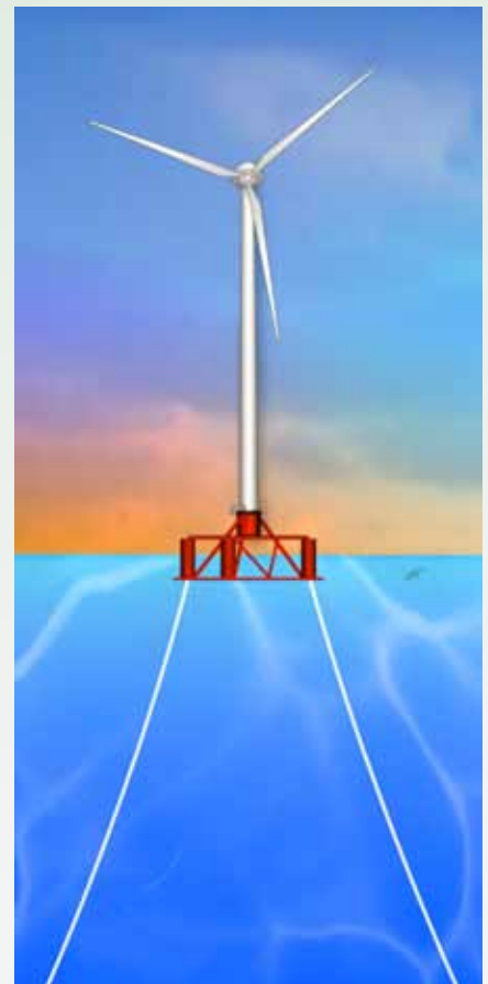
Figure 2 A Floating Semi-Submersible Will Be Analyzed in OC4 Phase II
