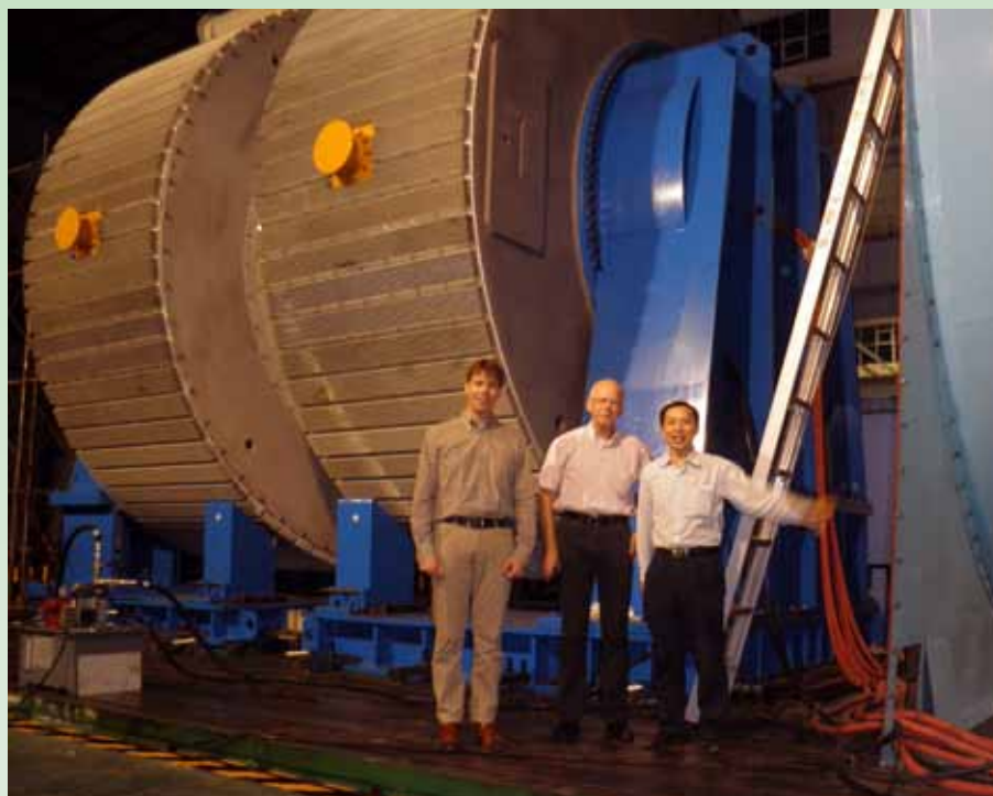
Figure 3 back-to-back test configuration 2 generators of XEMC-Darwind 5-MW, direct-drive, permanent-magnet generator
