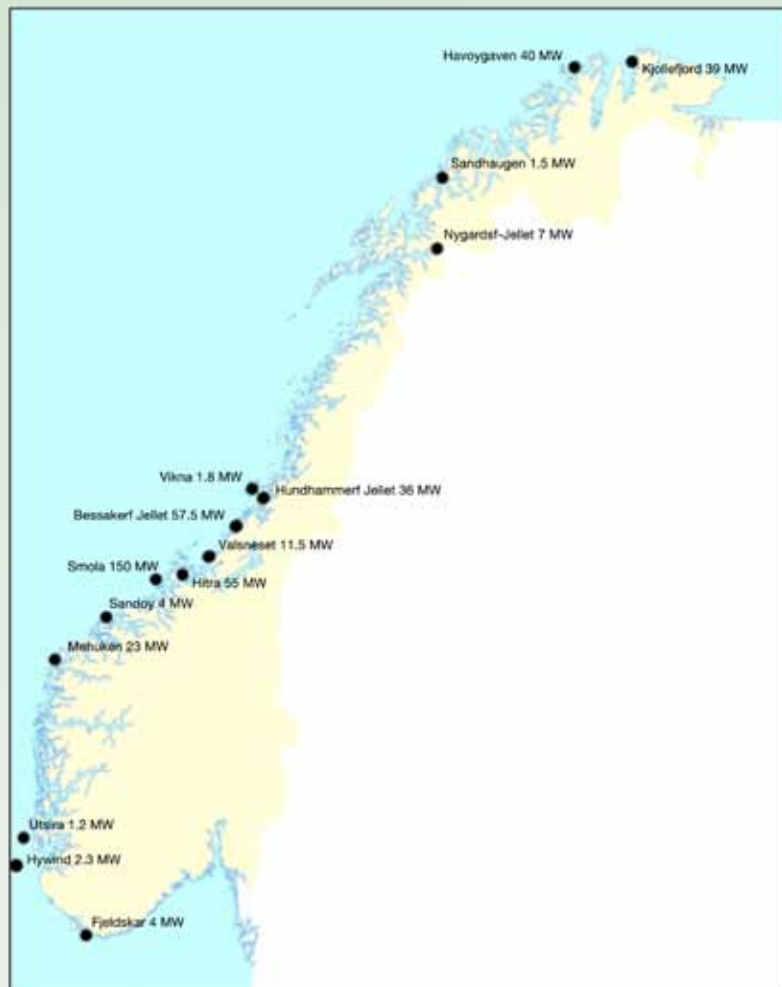
Figure 3 Location of wind power installations
