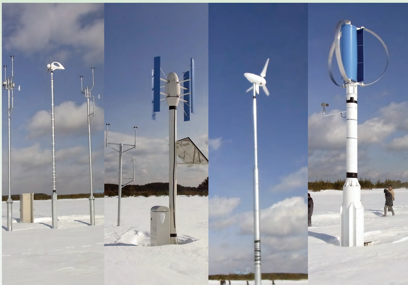
Figure 3. Field test site for small wind turbines in Rakkasho, Aomori (From left to right, Nasu Denki-Tekko "Aura 1000", Sinfonia Technology "V-II WK18-20", Nikko "NWG-1K", Mayekawa "MDS-01A") (Photo credit: HIKARUWIND.LAB)
