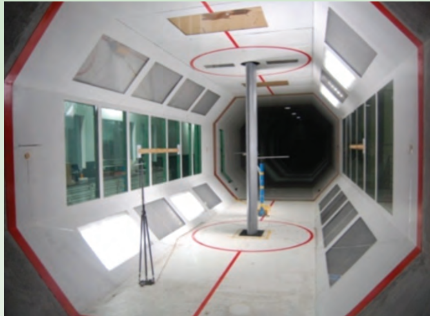
Figure 2. Airfoil test in the China Aerodynamics Research and Development Center, 4-m by 3-m wind tunnel
