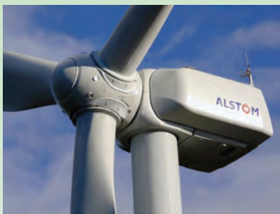
Figure 2. Large wind turbines commissioned at Energy Department-supported test sites in 2011. Left to right: Clipper Liberty 2.5-MW; Gamesa G97 2-MW Class IIIA; Alstom 3-MW Eco 100
