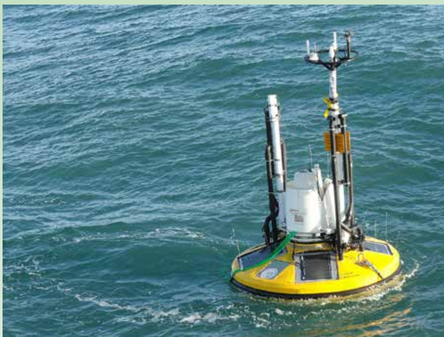
Figure 4. The Met Ocean Buoy with lidar being developed under the FLOW program
