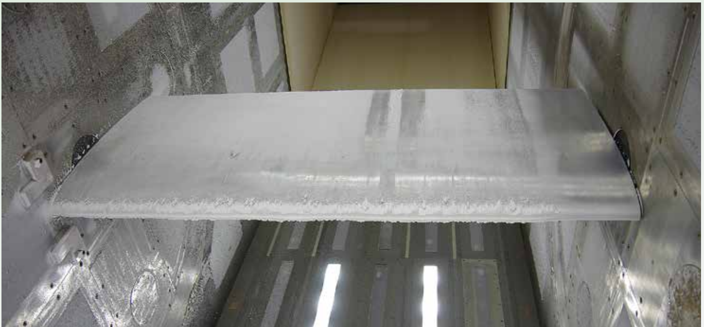
Figure 2. Test section of icing wind tunnel
