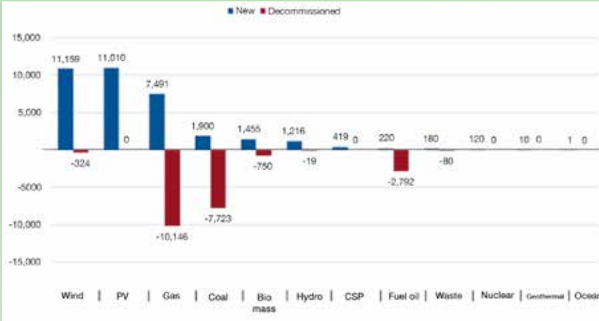
Figure 4. New installed power capacity and decommissioned power capacity in MW (Source: Platts Powervision and EWEA)
