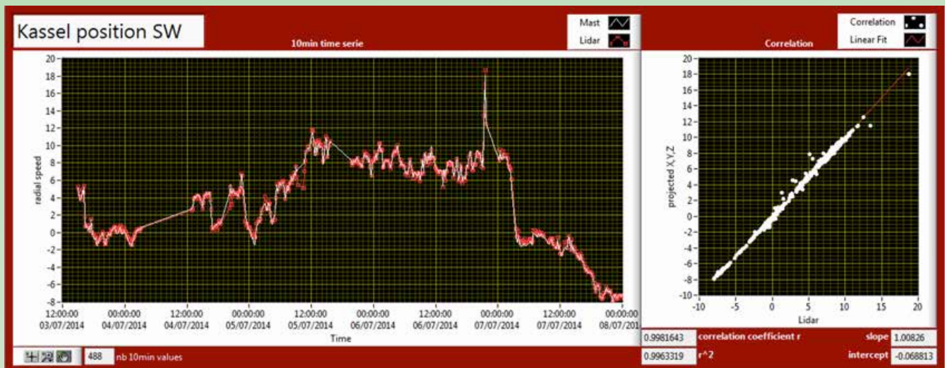
Figure 1. The 10-minute average of the radial wind speed and projected radial wind speed
