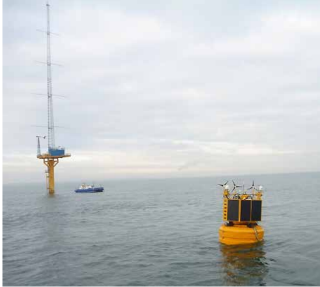
Figure 5. FLiDAR floating lidar system (Source: www.leosphere.com/products/floating/flidar-floating-buoy-lidar )
