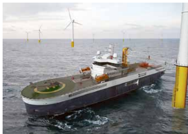
Figure 3. Z-bridge, a newly developed transfer system enabling transfer of goods and workers in wave heights up to approximately 3 m
