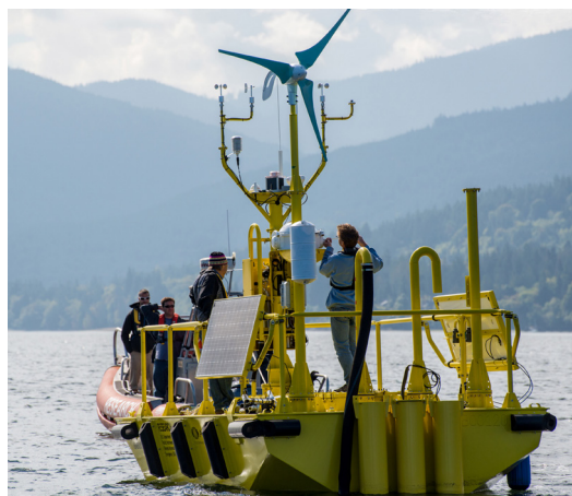
Figure 2. Lidar buoys like this one hold an array of advanced research equipment that can assess the energy potential of offshore wind sites and accelerate permitting. (Photo credit: Pacific Northwest National Laboratory)
