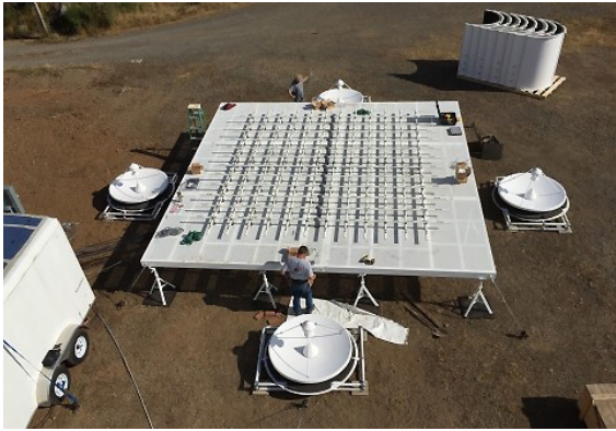
Figure 3. One of the new radar profilers installed along the west coast (Photo credit: Pacific Northwest National Laboratory)
