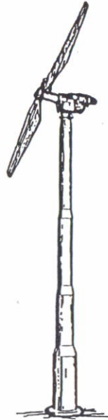
150 kW 150 ft tower height 70 ft rotor diameter
