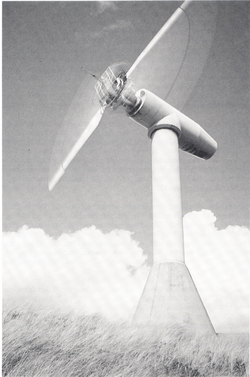
Figure 2.6.6 The FLEXHAT rotor mounted on the 25 m experimental wind turbine of ECN, Petten. The test concept is designed and engineered by Stork Product Engineering in cooperation with ECN. The test programme will be concluded in the first half of 1993. (Photo: Jos Beurskens).
