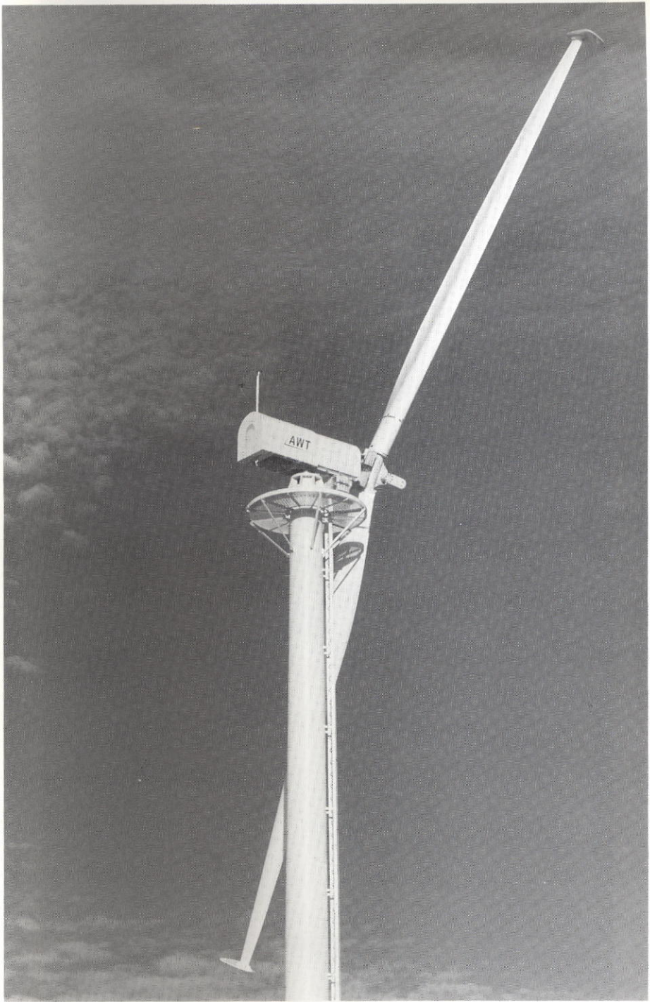
Figure 2.11.1 The 275 kW/26 m rotor diameter AWT-26, manufactured by Advanced Wind Turbines, Inc.
