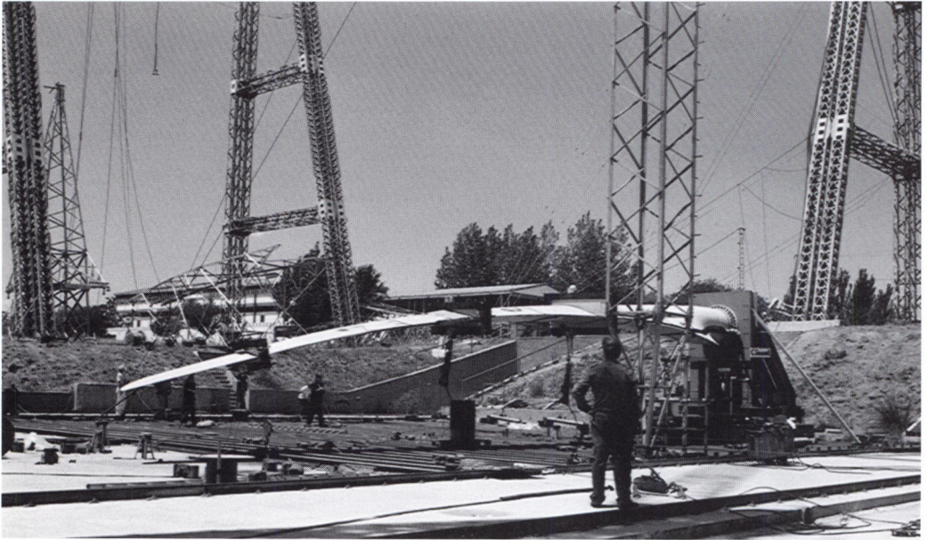
Figure 4. Static strength test (blade length 41m) SFAT project.
