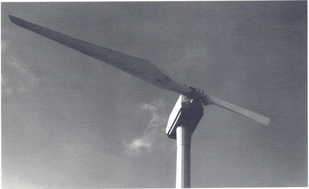
Figure 3. Closer view of the 350 kW M30-S2 machine. This model is the latest issue of Riva Calzoni's single-bladed series.
