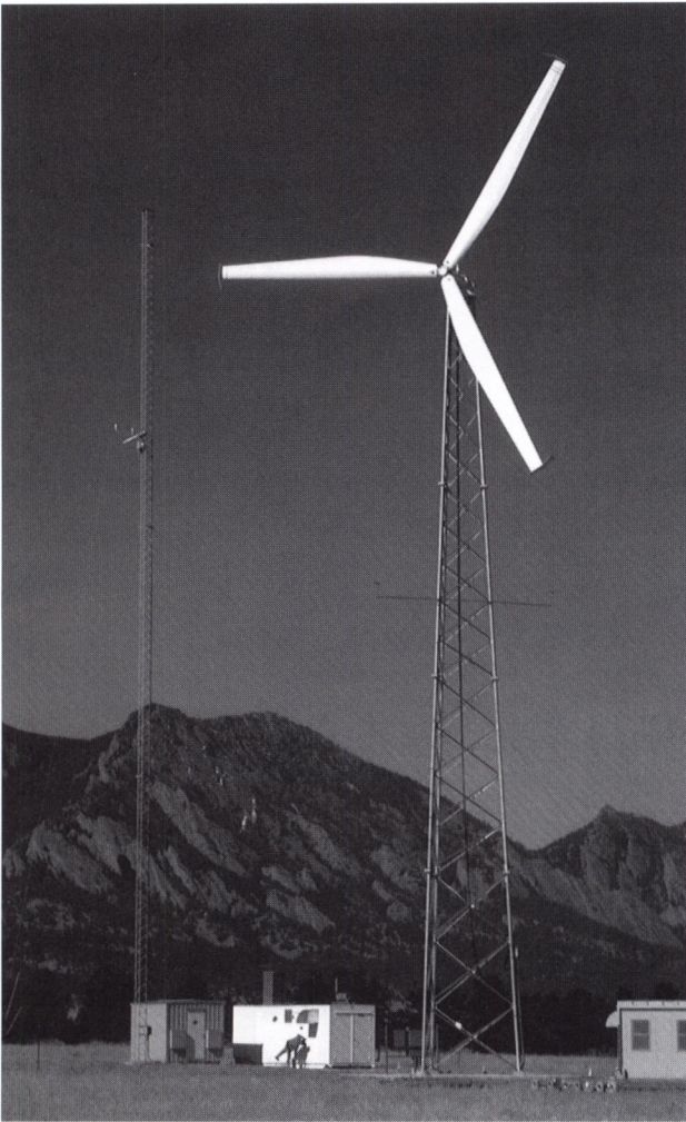
Figure 3. AOC 15/50, 50 kW turbine with 15 m rotor diameter being tested in wind/diesel applications at the National Wind Technology Center near Golden, Colorado.
