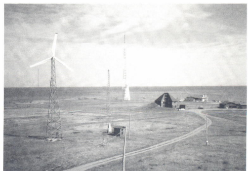
Figure 4.1 The AOC 15/50 turbine being tested at the Atlantic Wind Test Site, Prince Edward Island, Canada
