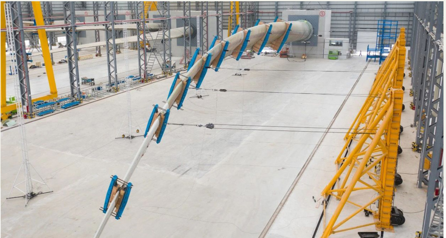
The first 102m long blade under full-scale test
