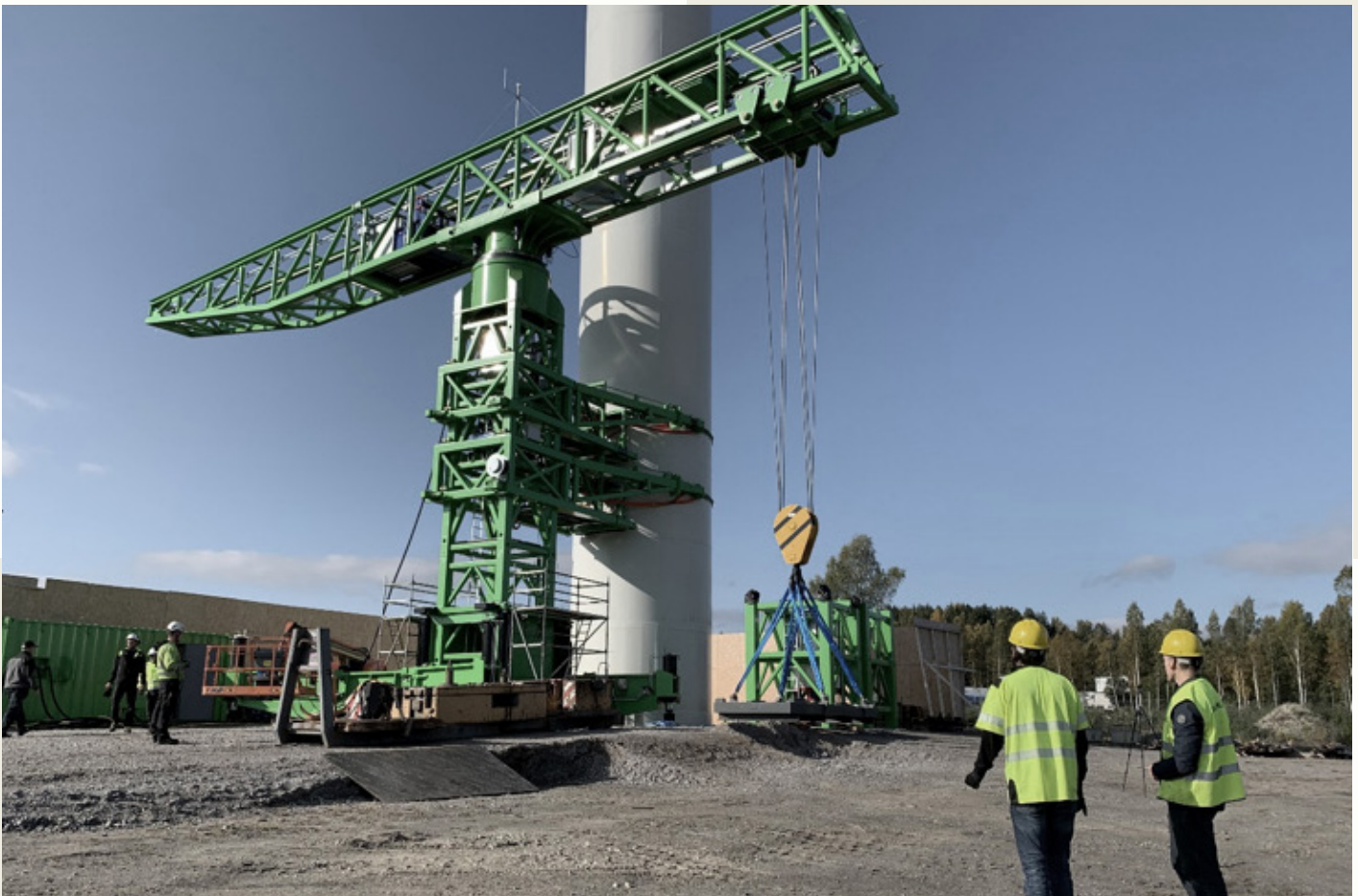
S&L Access Systems, Salamander Quick Lift Crane prototype. (Source: S&L Access Systems)
