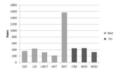
Figure 4-5: Icing hours from various ice detection methods showing the relative humidity and temperature method significantly over-estimates icing duration compared to all other methods tested [19].
