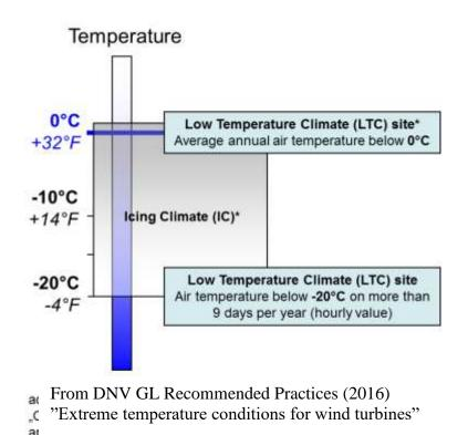
Figure 3-1: Low temperature and icing climate with respect to ambient temperature.
