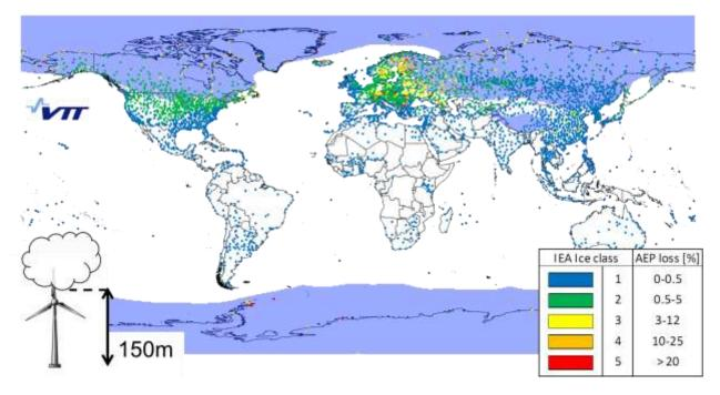
Figure 0-1: Global icing and low temperature (in blue) map [2], [3]
