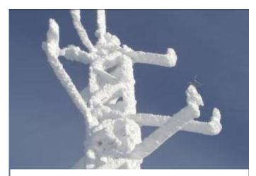
Figure 4-2: The impact of ice build-up on mounting hardware and sensors must be considered to ensure the accuracy of wind speed and direction measurements. Photo credit: TMV2 Murdochville, TechnoCentre éolien.
