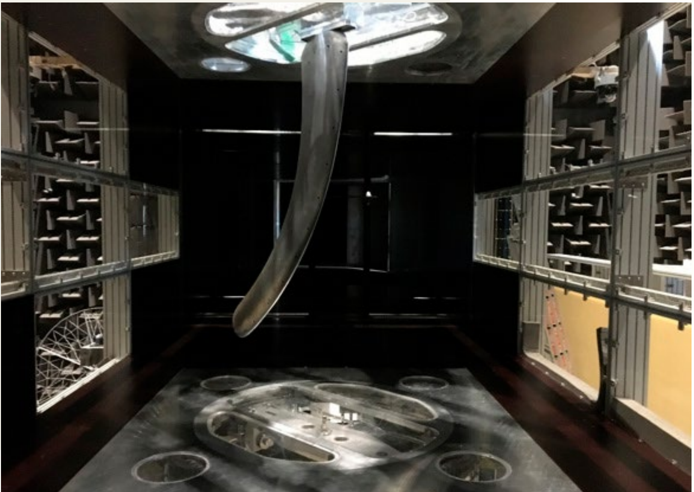
Fig. 1: Swept blade tip measured in a DTU-PLC wind tunnel.
