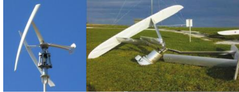
Figure 3: Damage caused by vibrations and at the Lichtenegg Research Park.
