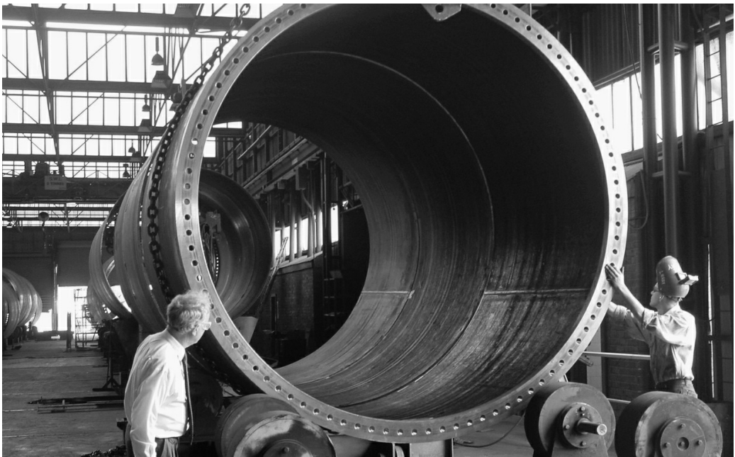
Figure 9.5 Manufacturing towers for Enercon turbines, Western Australia
