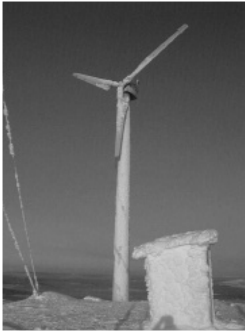
Figure 6.2 This Pyhäntunturi test station in Finland has been the base for developing blade-heating systems for wind turbines
