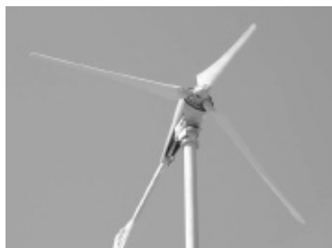
Figure 14.9 The new "Miniwind" 15-kW wind turbine developed by Enel WindPower. It features a 3-bladed, 8-m-diameter, variable-speed rotor and a permanent-magnet synchronous generator connected to the network through an a.c./d.c./a.c. converter. Cut-in wind speed is 3 m/s, rated speed 10.5 m/s, cut-out speed 25 m/s.
