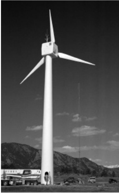
Figure 23.6 100-kW, cold-weather turbine built by Northern Power Systems under test at the NWTC near Boulder, Colorado
