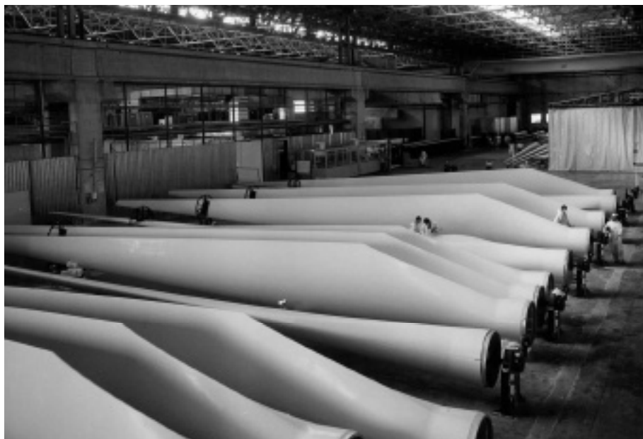
Figure 14.7 IWT facility-Taranto V-47 blades production (photo Carmine La Fratta).
