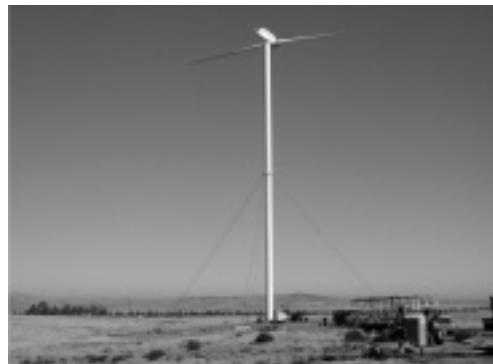
Figure 23.5 Wind Turbine Company's 500-kW, 48-m in diameter turbine under test at a Los Angeles Department of Power and Water site near Fairmont, California
