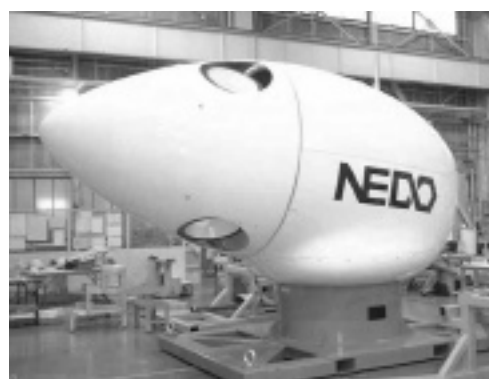
Figure 15.2 Nacelle components of a 100-kW wind turbine for remote islands
