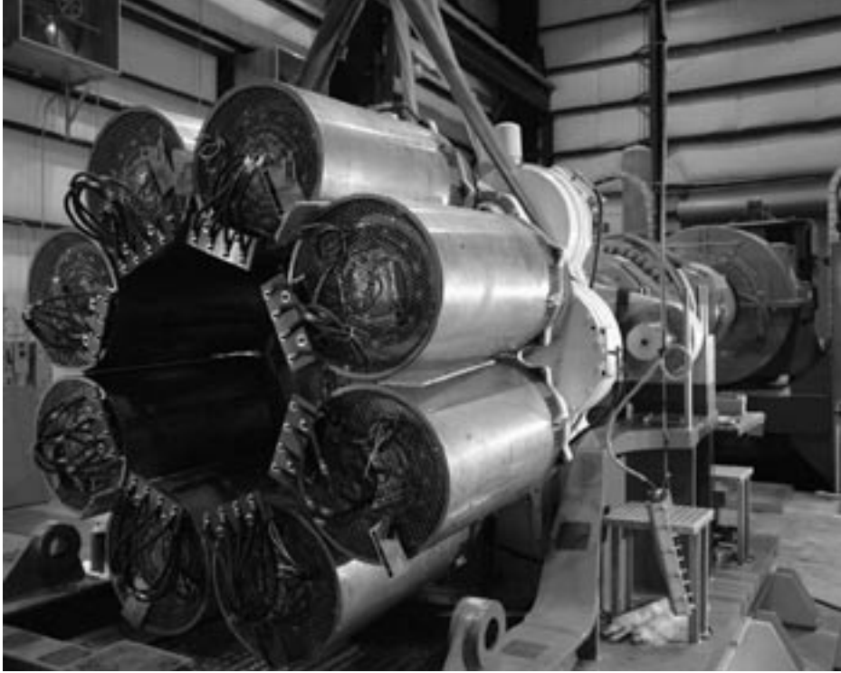
Figure 21.7 Clipper Windpower developed a new, 8-generator, 1.5-MW-to-2-MW drivetrain
