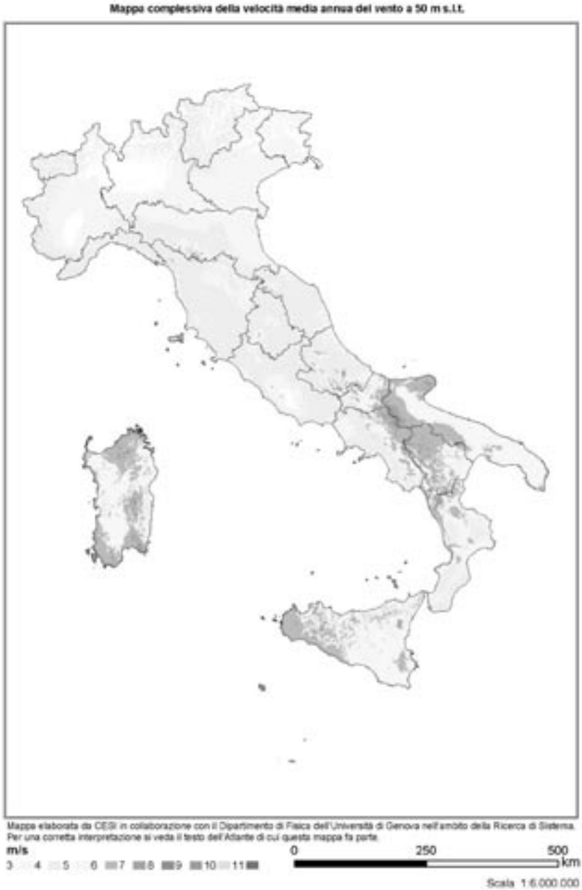
Figure 11.6 Overall synthesis map of annual mean wind speeds at 50 m above ground, taken from the Wind Atlas of Italy
