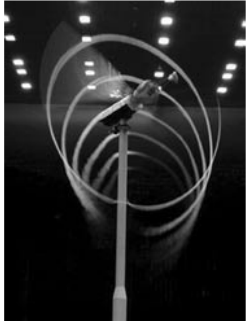
Figure 2.6.1 NREL UAE in NASA Ames 80-foot by 120-foot wind tunnel
