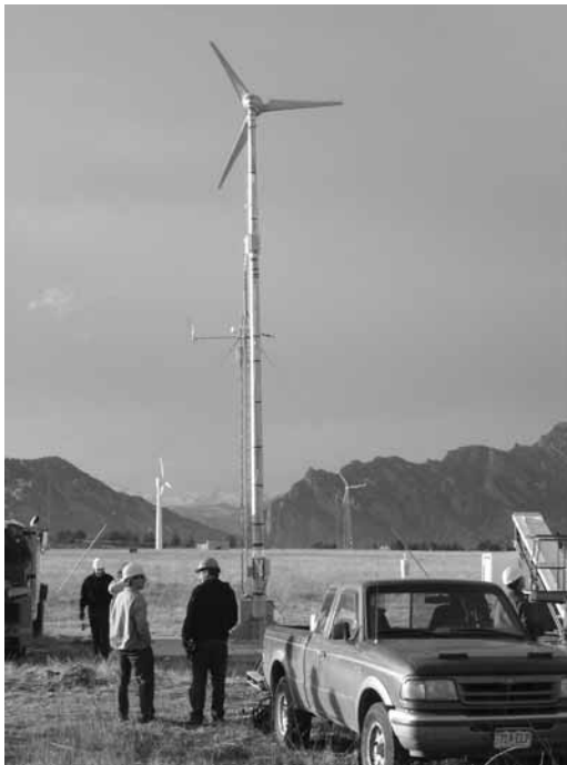
Figure 5 The Southwest Windpower Storm prototype turbine was installed at NREL in December 2004 for field-testing.
