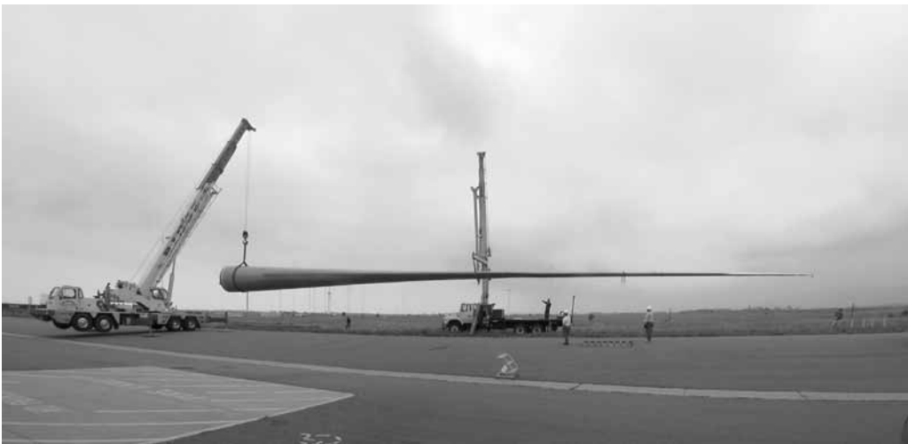
Figure 7 NREL receives a 45-m blade sent by TPI Composites for testing.
