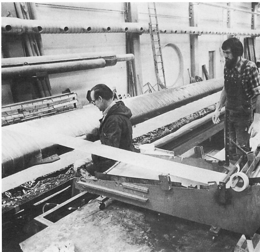
Manufacture of D-spar of glass-fibre plastic with the rovings all laid longitudinally on a rotating mandrel.
