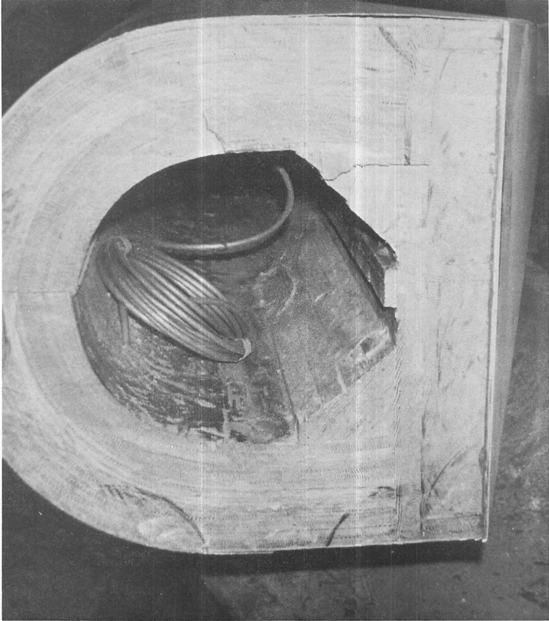
ROOT END OF 60 FOOT WOOD BLADE AFTER ROUGH TRIM CUT. "D" THICKNESS 4.75 INCHES
