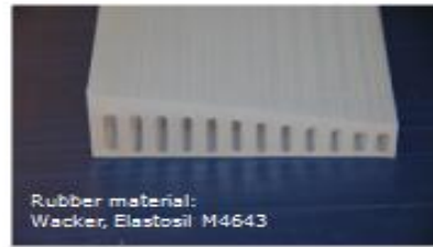
Geometry of the voids and the wall thickness were optimized to achieve a lower and more uniform stress level
