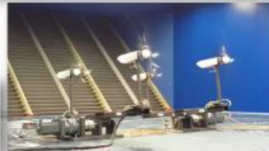
▼ Power effect by misalignment ( \theta = 10 deg)
