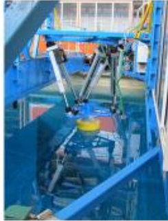
View of the hexapod configured for forced oscillations tests (Source: Ifremer)
