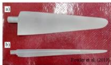
Fig. 1 Images of a) redesigned, thrust-matched blade and b) original geometrically-scaled, NREL 5 MW reference wind turbine blade.
