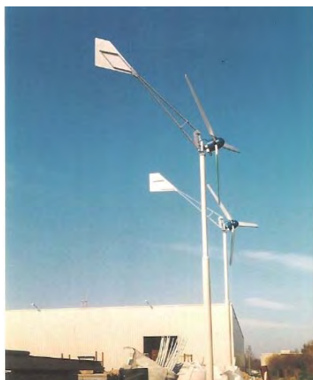
Fortis Montana Horizontal axis windturbine 5 m rotor diameter
