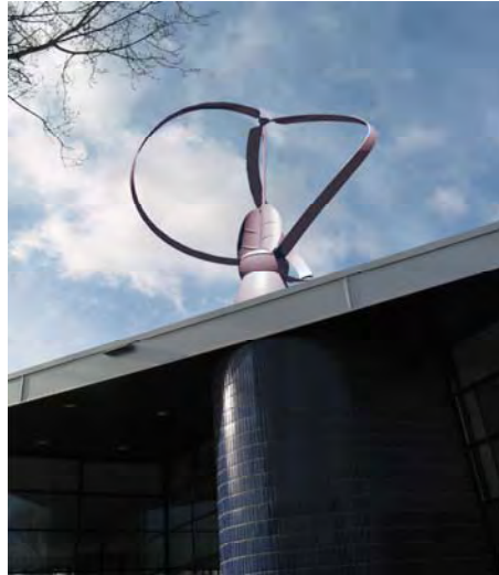
NEOGA Ecofys Vertical axis wind turbine Darrieus rotor 3 m diameter
