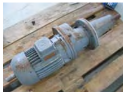
Generator with drive train
