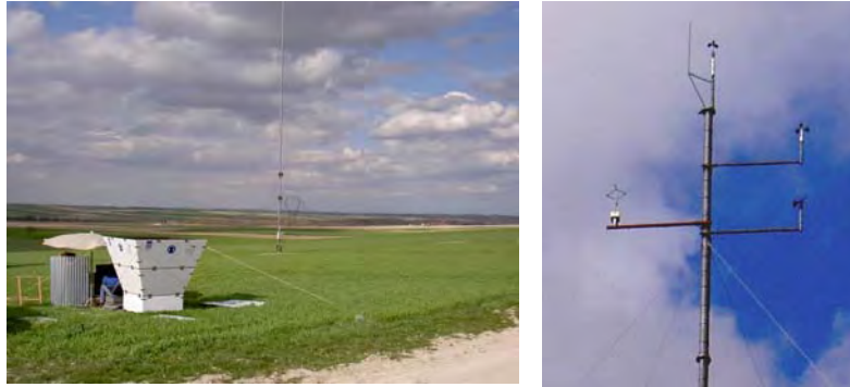
Instruments: SODAR, cup anemometer, wind vane and 3-D sonics
