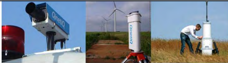
Figure 3. Stages of evolution of the ZephIR lidar. Figure 3a shows the lidar head mounted on the nacelle of a Nordex N-90 wind turbine. Figure 3b shows prototype ground-based wind profiler at Risø wind energy test site, Høvsøre, Denmark. Figure 3c shows the ZephIR production model deployed in the field
