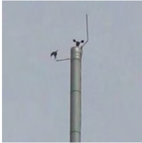
Detail of the top mast anemometer
