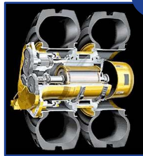
AC/DC – Compound Planetary 1,200 Hp (900 kW) motoring 2,000 Hp (1.5MW) retarding
