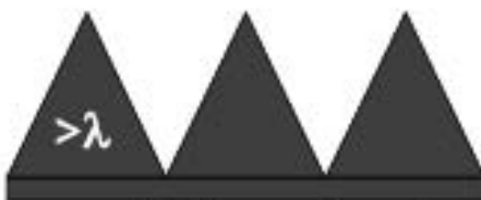
pyramidal foam absorber
