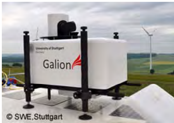
Fig 1: Scanning Lidar system at a complex site in Southern Germany [SWE, University of Stuttgart]
