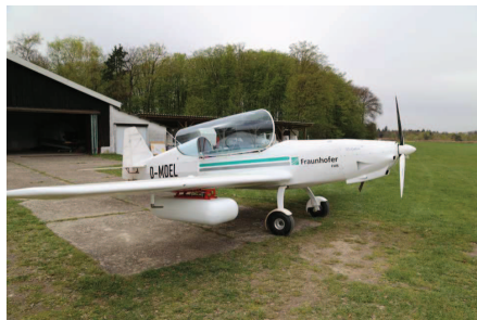
Integration of a measurement receiver including flight recorder into the FHR experimental airplane „Delphin“
