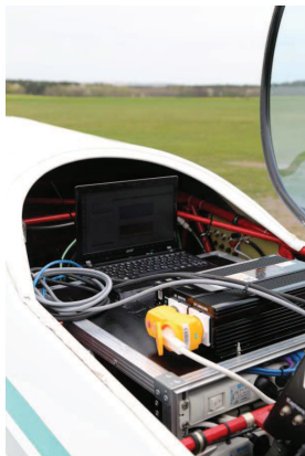
Integration of a measurement receiver including flight recorder into the FHR experimental airplane „Delphin“
