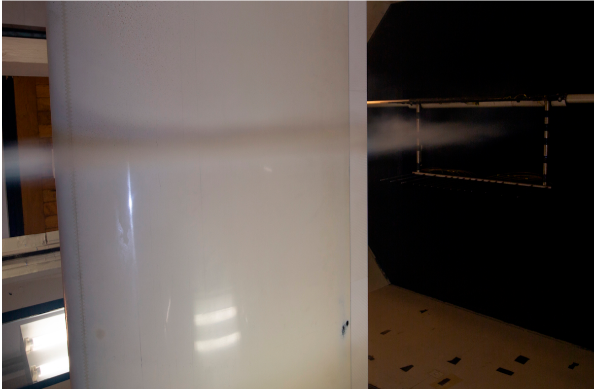
Photo 2. Part of a wind turbine blade with MuteSkin blade extension in wind tunnel test with microphone array.
