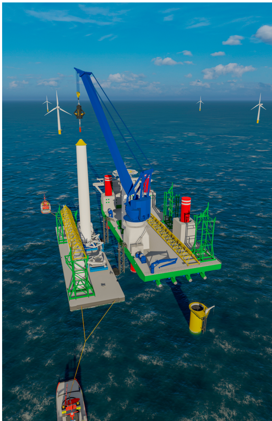
Figure 6. Barge alongside jack-up vessel lifting a mast (Source: Barge Master).
