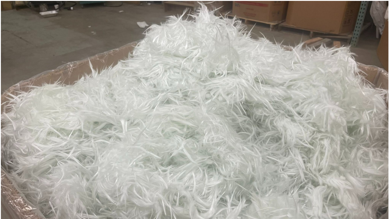
Figure 1: With the help of WETO funding, Carbon Rivers has achieved 99.9% recycled glass fibre purity from different end-of-life waste streams like wind turbine blades. The high purity opens the potential for remelting—allowing recycled glass fibre to be incorporated into virgin fibreglass, thereby closing the material loop and creating a circular economy. Photo from Carbon Rivers.
