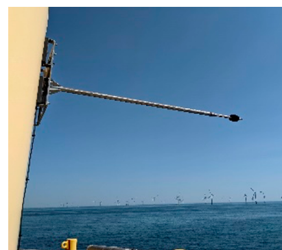
Figure 2: Microphone test set-up at the Rentel offshore wind farm.
