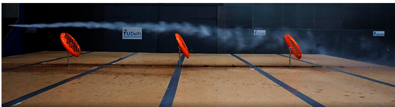
Image 2: Disc experiments in the wind tunnel at the TU Delft, pulling air downwards (TouchWind).
