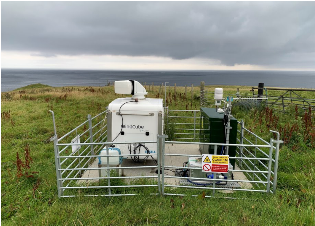
Figure 3: Scanning lidar installation – one device of a pair in a dual setup – at nearshore site. Photo credit: Fraunhofer IWES.
