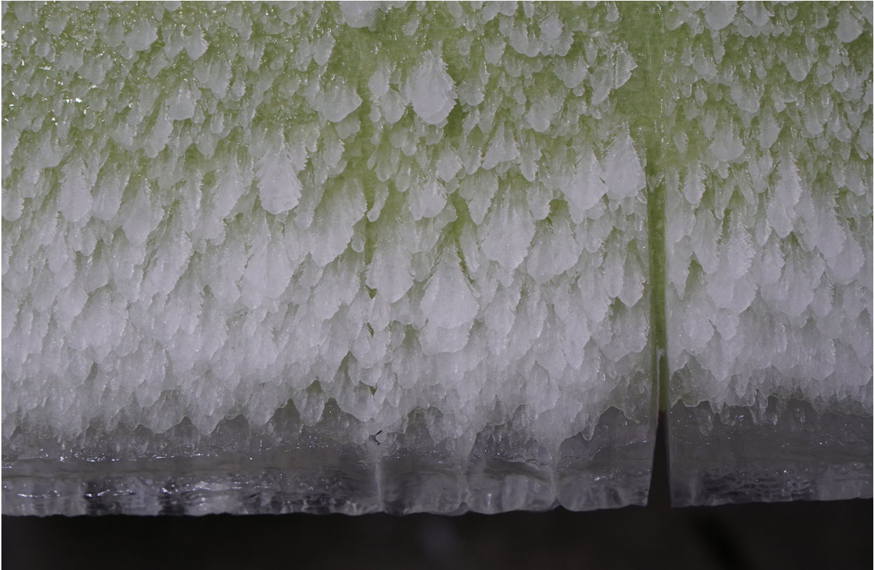
Photo 1: Ice accretion on a blade profile in an icing wind tunnel.
