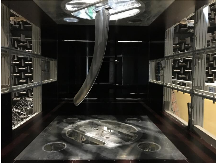
Figure 5 - Blade tip measured in DTU PLC wind tunnel
