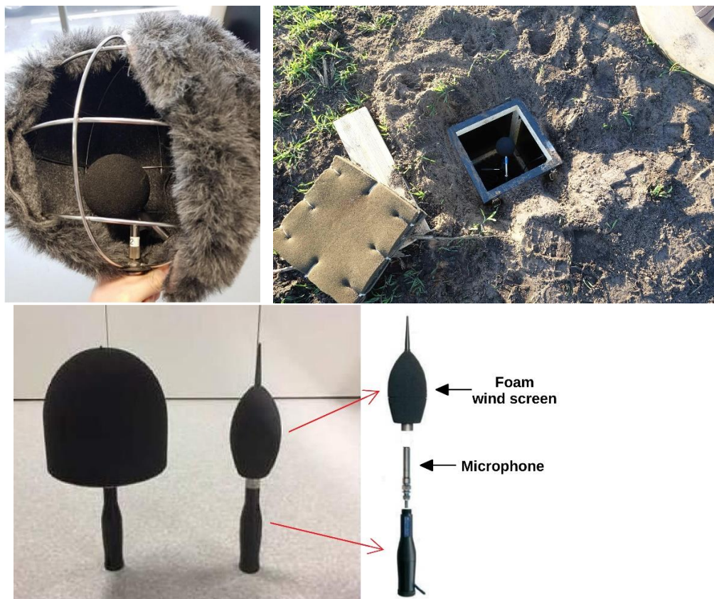
Figure 3 – Top left picture: Outer fur wind screen, with inner foam wind screen for extra protection, shielding a microphone from the wind for outdoor noise measurements [Source: FORCE Technology, Denmark] - Bottom picture: Foam outer (left) and inner (middle) wind screens with the inner assembly contains the microphone (right) [Source: Norsonic AS, Norway] – Top right: Microphone (with foam wind screen) placed in a wooden box at the ground level to minimize wind effect [Source : Blumendeller2020]
